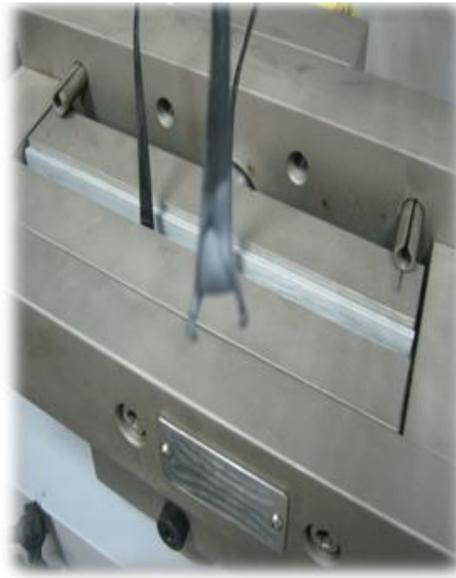
**Figure 7:** Geogrid Rib Rupture
