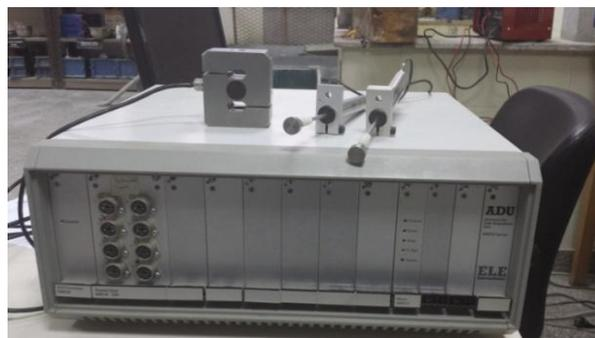
Figure 13: Data acquisition unit
