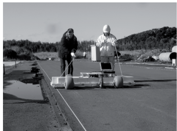
Figure 9. Data acquisition with the YAKUMO system on the airport-runway model at the Nobi experimental site.
