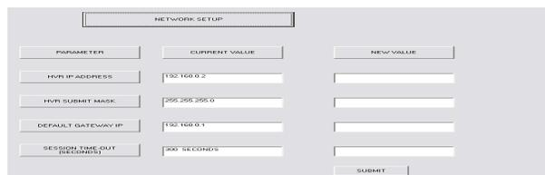
Fig. 11 Sample screen shot of the VDR network setup page
