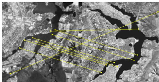
Fig.2 Matching points results from first level SIFT.
