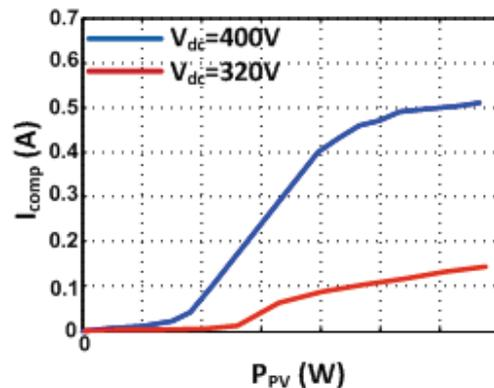
Fig. 5. Mapping between  $P_{PV}$  and  $I_{comp}$
