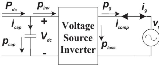
Fig. 2. Power flow at the DC and AC sides of the inverter
