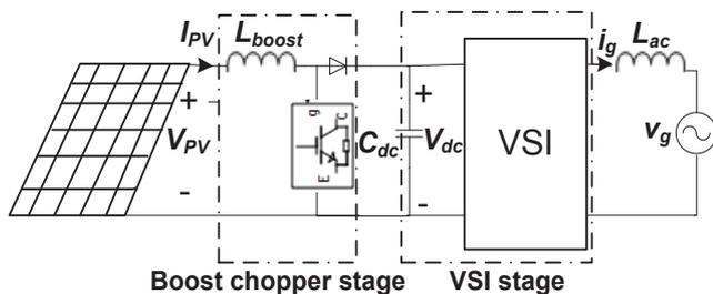
Fig. 1. PV-grid connected system under consideration
