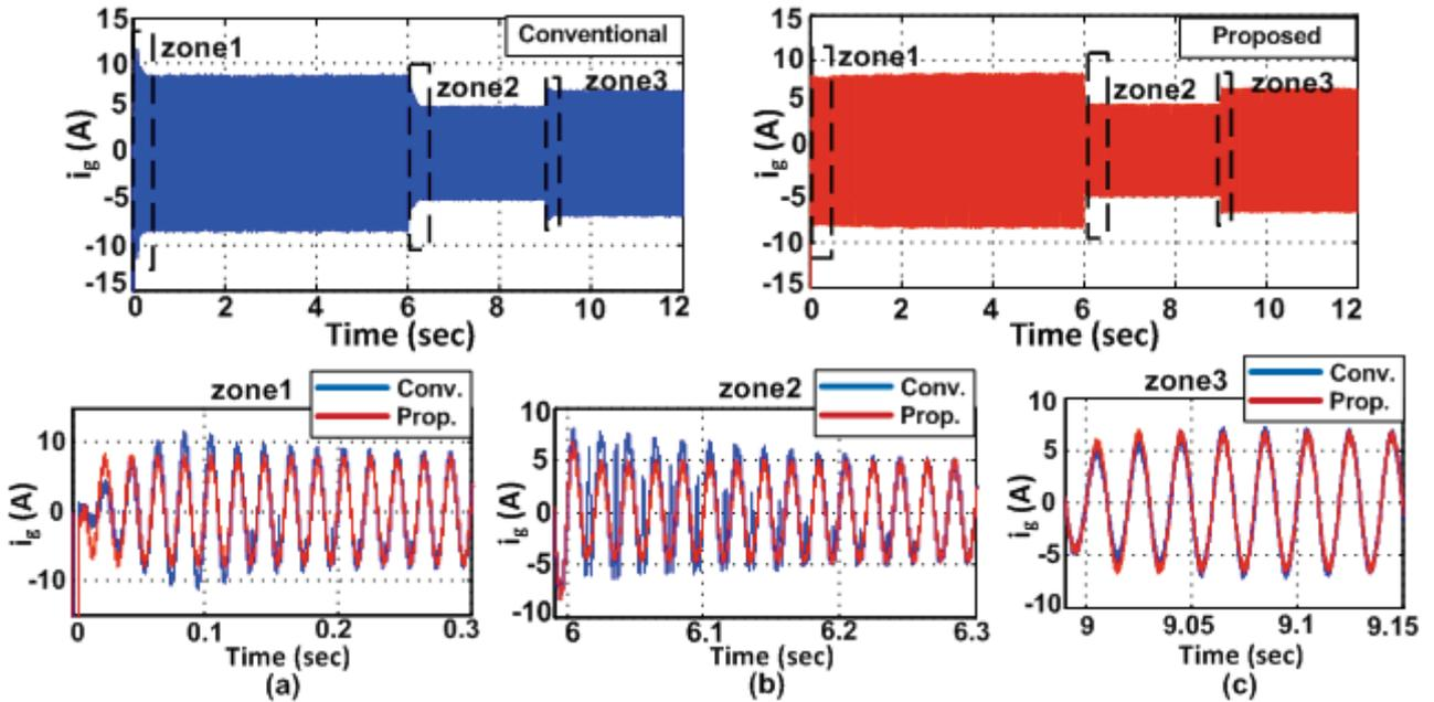
Fig. 9. Grid current for conventional and proposed techniques during: (a) Start-up, (b) First step change, (c) Second step change
