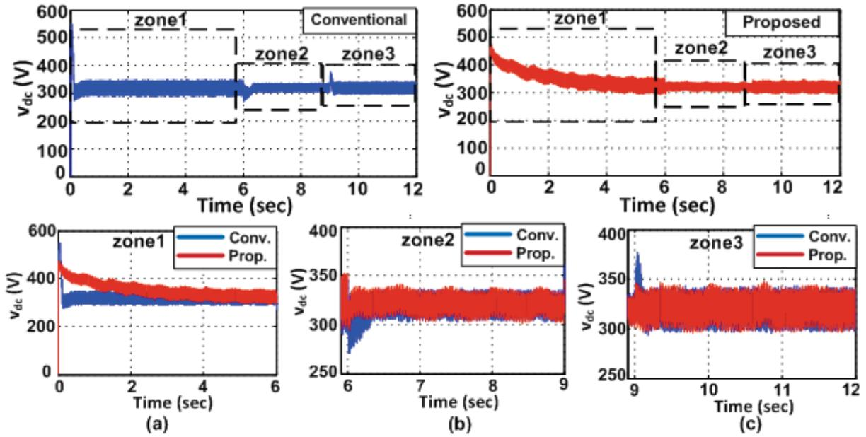
Fig. 8. DC-link voltage for conventional and proposed techniques at variable irradiance levels; (a) 1000 W/m<sup>2</sup>, (b) 600 W/m<sup>2</sup>, (c) 800 W/m<sup>2</sup>
