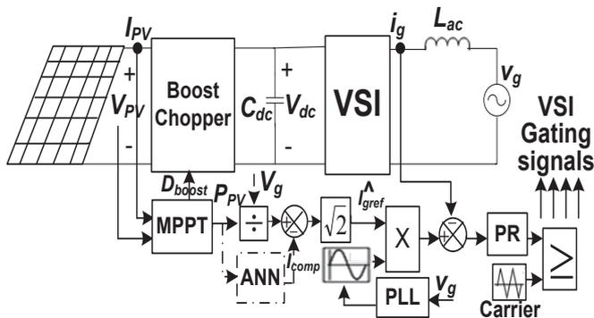
Fig. 4. Proposed sensorless control technique scheme
