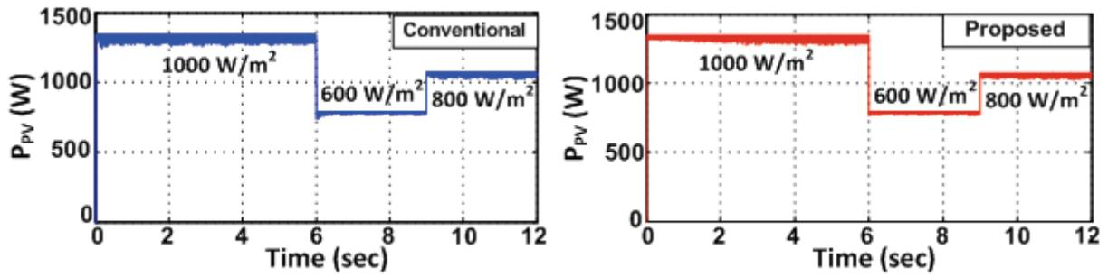
Fig. 7. Maximum power extracted from PV string using conventional and proposed techniques at three different irradiance levels
