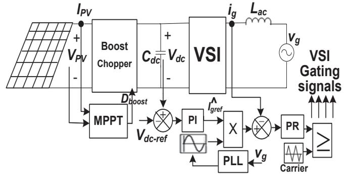
Fig. 3. Conventional control technique scheme
