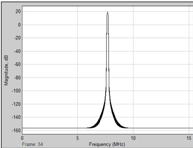
Fig.6 Spectrum of IF signal after Sub-sampling (7.68 MHz)
