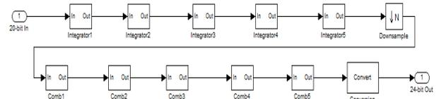
Fig.2 Architecture of CIC filters
