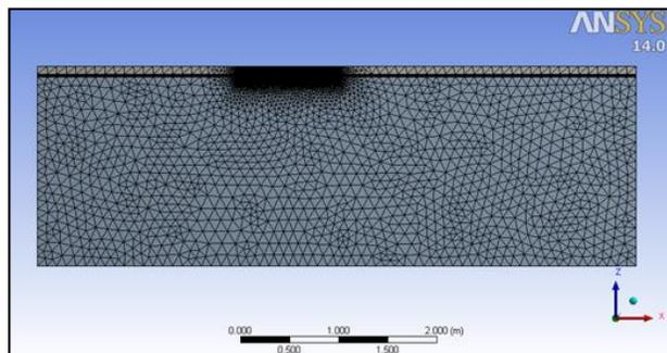
Figure 3(a). Grid1 with prism layers in the free surface region and on Wigley hull (total number of mesh elements is 1,598,573 tetrahedral elements)
