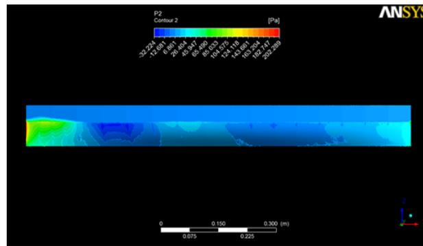
Figure 10(b). Dynamic pressure contours on the Wigley hull at  $Fr = 0.267$  ( $V = 0.8363$  m/s) for Grid2.
