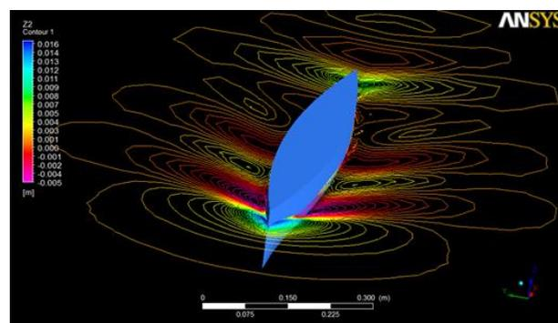
Figure 8(a). Grid1 wave contours around Wigley hull at  $Fr = 0.267$  ( $V = 0.8363$  m/s).
