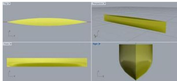
Figure 1. Different plan views for the Wigley hull.
