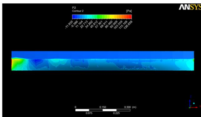
Figure 9(b). Dynamic pressure contours on the Wigley hull at  $Fr = 0.2$  ( $V = 0.6264$  m/s) for Grid2.
