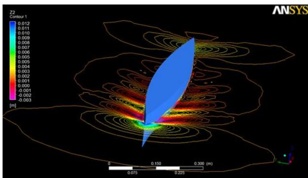
Figure 7(a). Grid1 wave contours around Wigley hull at  $Fr = 0.2$  ( $V = 0.6264$  m/s).
