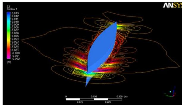
Figure 7(b). Grid2 wave contours around Wigley hull at  $Fr = 0.2$  ( $V = 0.6264$  m/s).
