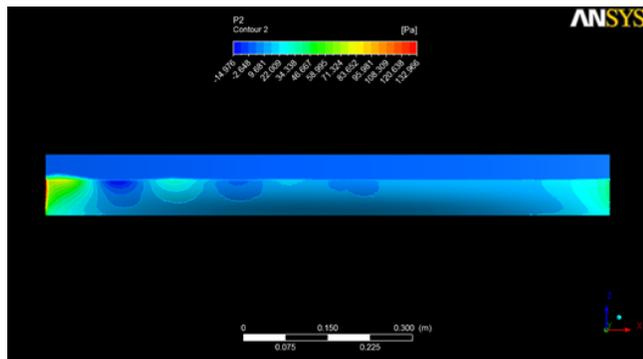
Figure 9(a). Dynamic pressure contours on Wigley hull at  $Fr = 0.2$  ( $V = 0.6264$  m/s) for Grid1.
