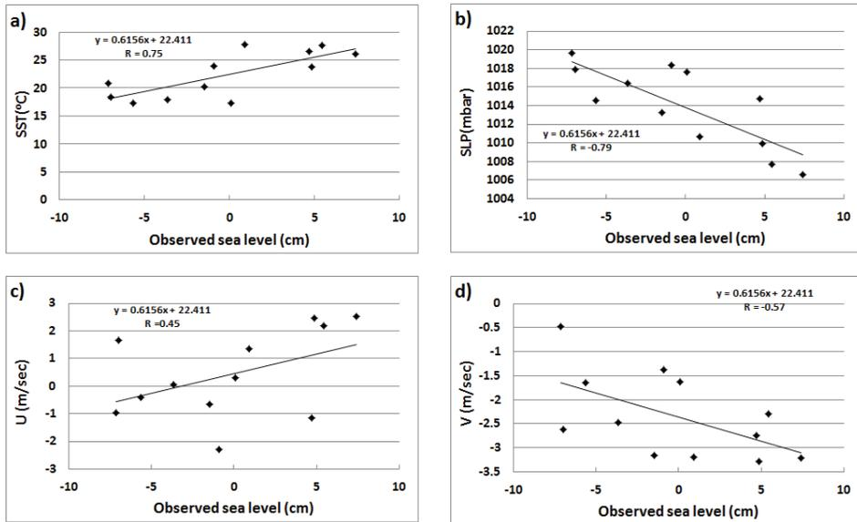
Fig. 6. The effect of monthly sea surface temperature (SST), mean sea level pressure (SLP), zonal wind (U) and meridional wind (V) on observed sea level off Port Said.
