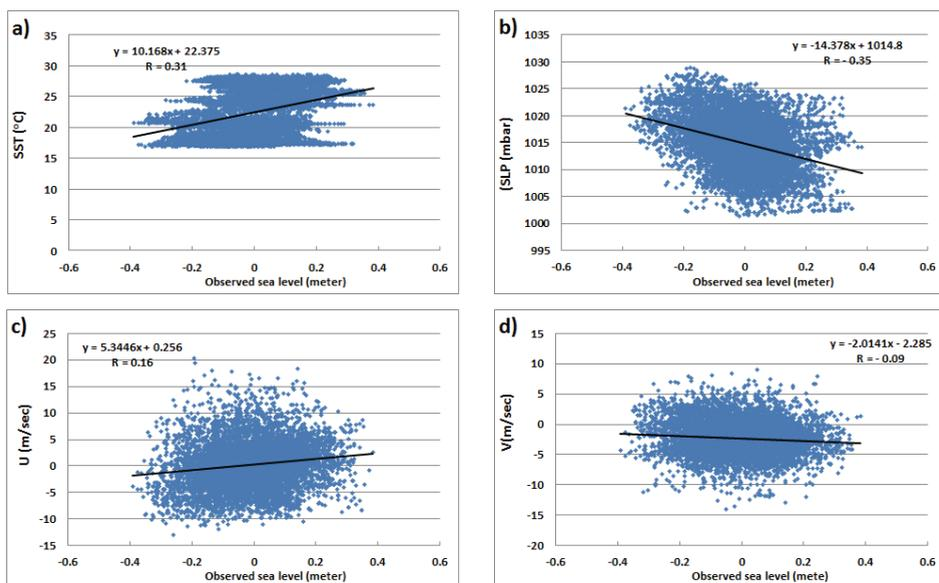
**Fig. 5.** The effect of hourly sea surface temperature (SST), mean sea level pressure (SLP), zonal wind (U) and meridional wind (V) on observed sea level off Port Said.
