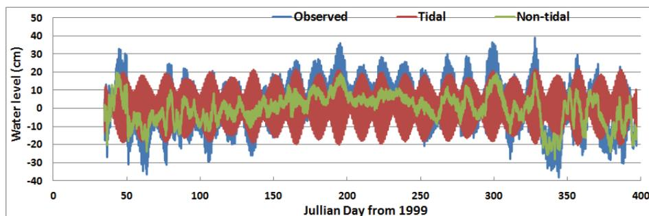
Fig. 3. Hourly observed, tidal, and non-tidal sea level off Port Said from February/99 to January/2000. (The run is based only on the important five tidal constituents).
