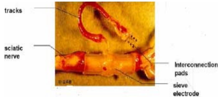
Figure 9: Implantable electrodes
