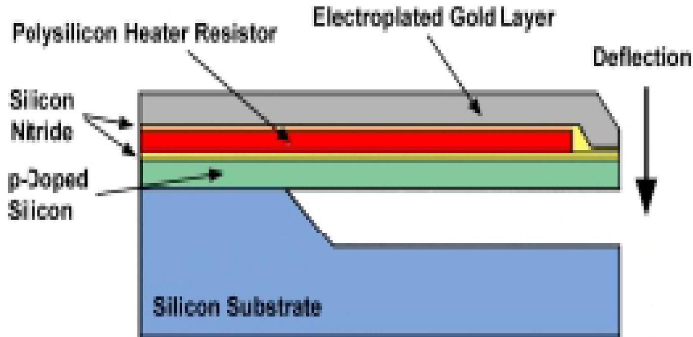
**This can be applied to a volume of fluid (liquid or gases) in sealed cavities with a thin membrane as a wall. By incorporating a heater the liquid can be heated causing it to expand and deform the membrane outwards. Large forces can be achieved using thermally actuated devices but power consumption can be high and it can take time for material to cool to its original activation state.**
