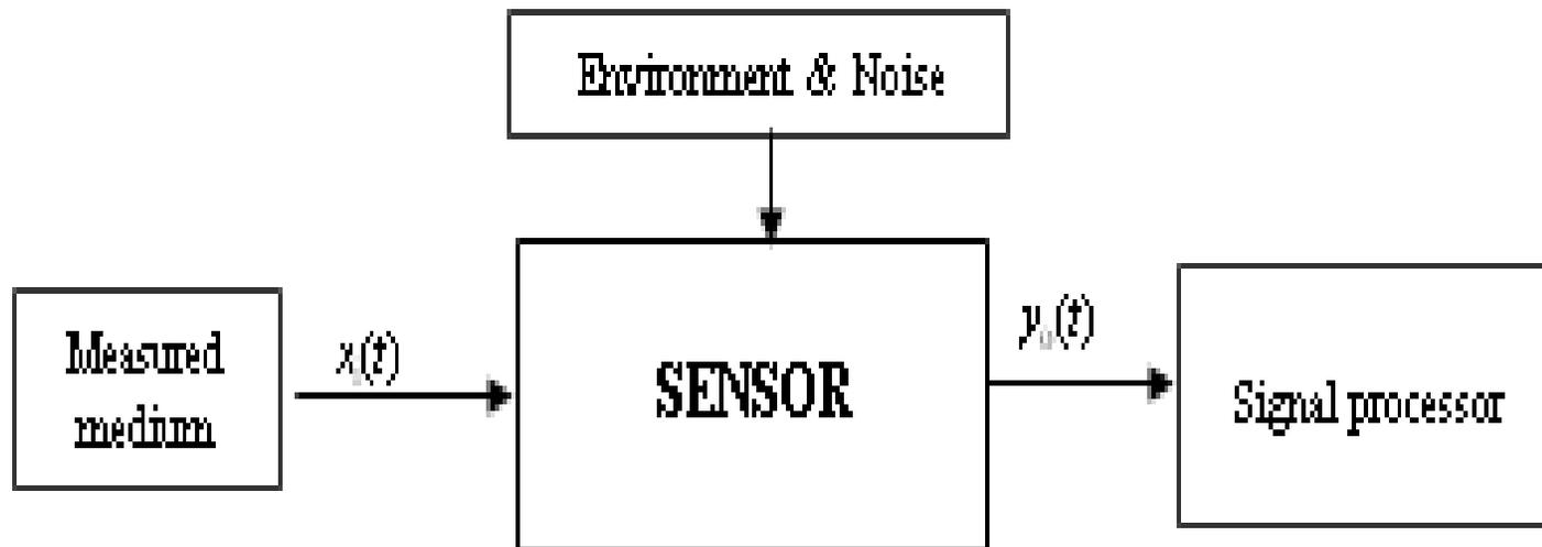
Figure1: Schematic representation of a sensor
