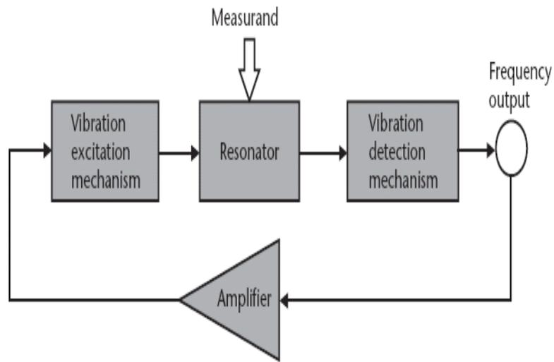
Block diagram of a resonant sensor.
