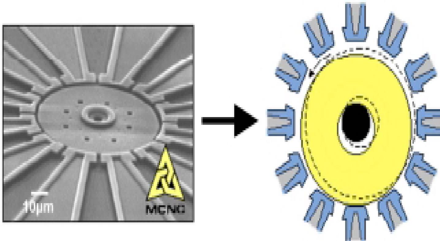
ii) **Piezoelectric actuation:** the piezoelectric effect can be used in both sensors and actuators. In piezoelectric actuation, the electrically induced displacement (or strain) is proportional to the applied potential difference. Despite small displacements, relatively high forces (in the region of tens of MPa) can be achieved using lower voltages than those required for comparable electrostatic actuation. It should be noted,
