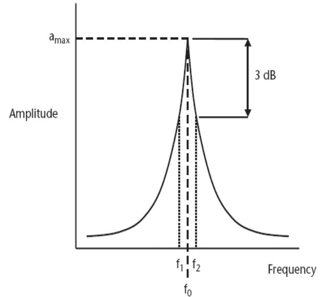
A typical characteristic of a resonant system.
