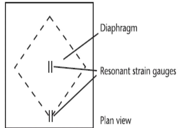
Druck resonant pressure sensor
