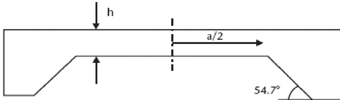
Anisotropically etched silicon diaphragm
