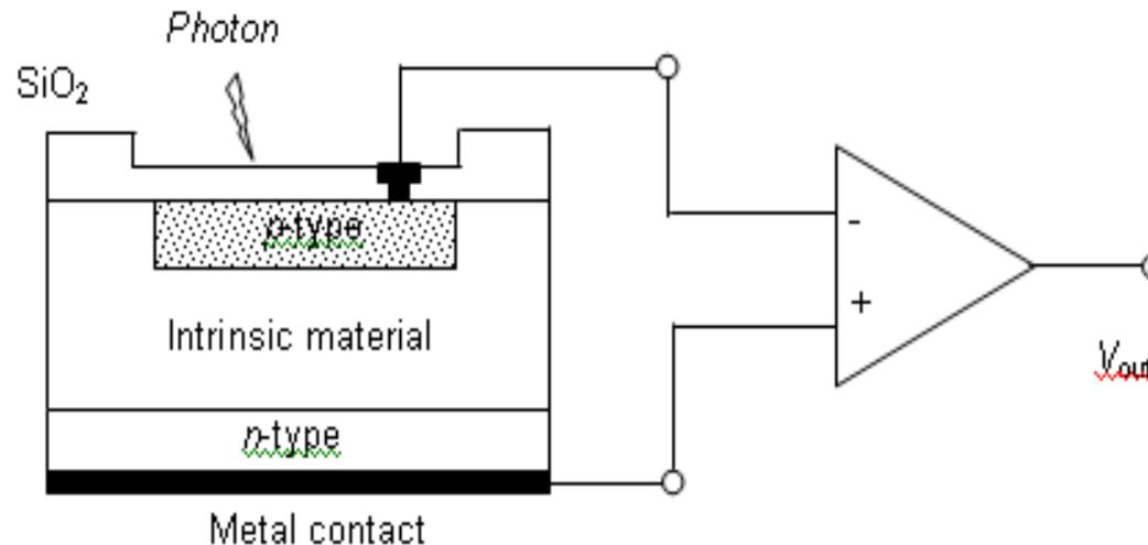
**Figure 4: Typical structure of a photodiode**
