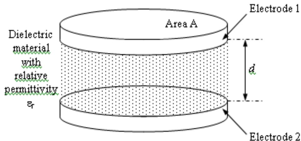
Figure 3: capacitive sensor
