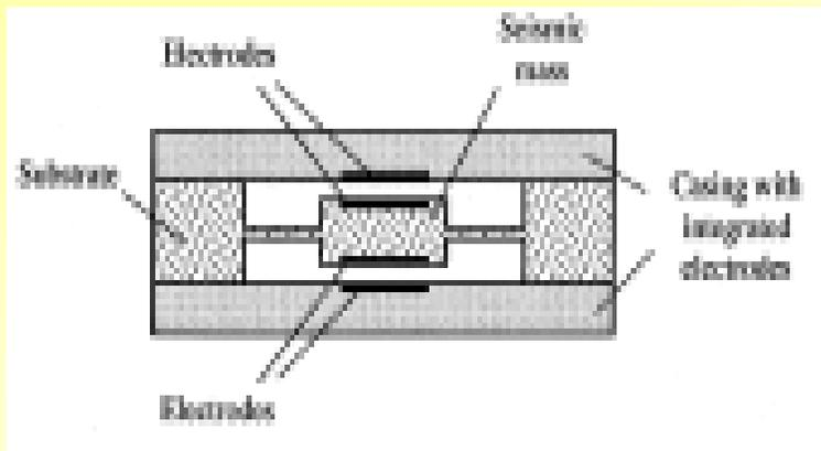
Capacitive measurement of acceleration.
