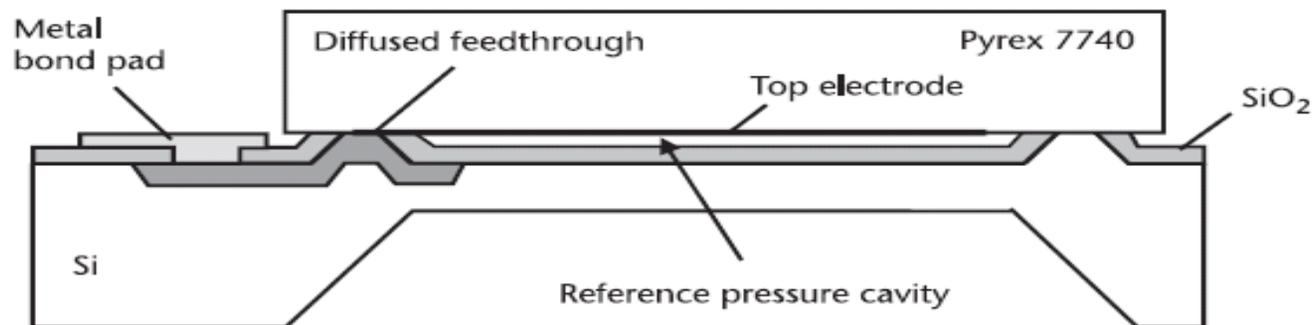
Early silicon/Pyrex capacitive pressure sensor
