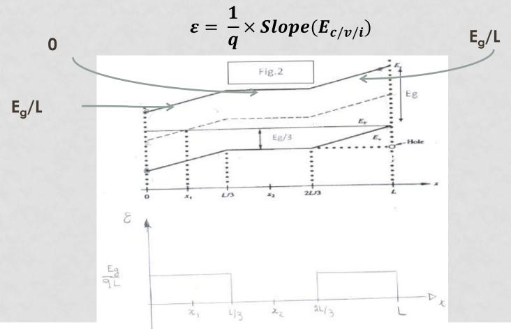
5. Draw the electrostatic potential inside the semiconductor
