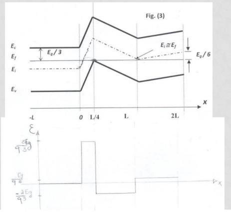
3. Sketch the electrostatic potential (V) inside the semiconductor as a function of x.
