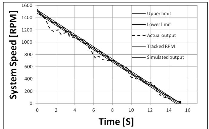
Figure.11 System response (Braking in 15 sec with a range  $\pm 20$  RPM)
