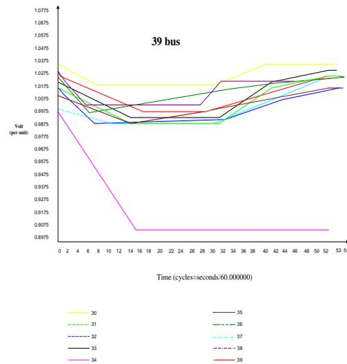
Fig. 11 Generators Bus Voltage after Applying AIS Development techniquemicro grid
