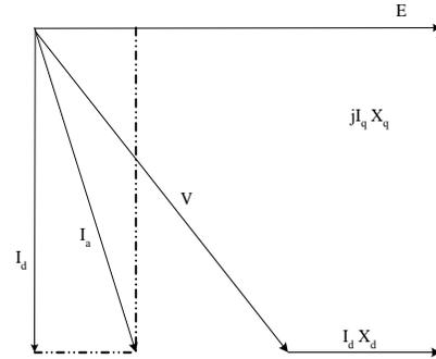
Fig. 1 Transient V-I phasor diagram
