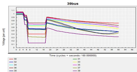
Fig. 10 Generators Bus Voltage for applying cascaded fault 21
