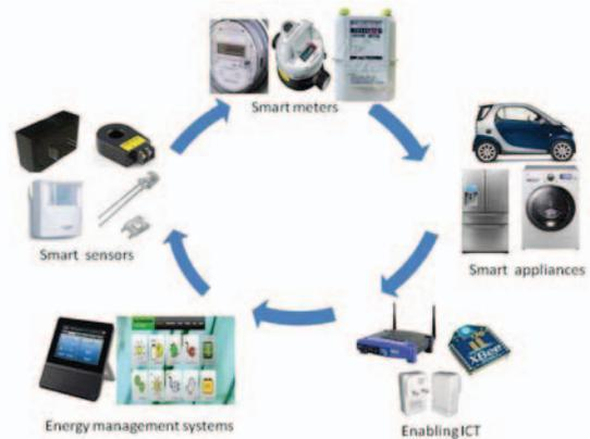
Fig.4: Fundamental components of home energy management system
