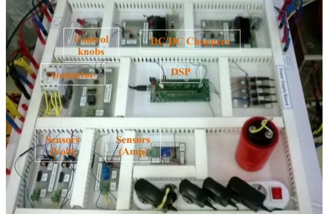
(b) Control setup with chopper and sensor circuits.
