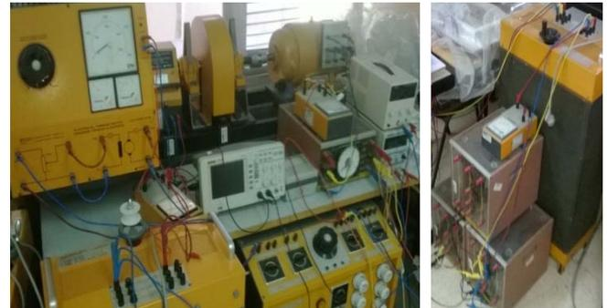
(a) Power setup with motored AC alternator, AC grid and load.
