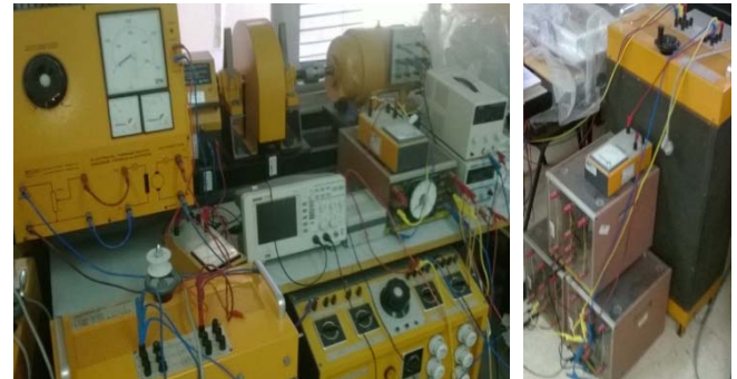
(a) Power setup with motored AC alternator, AC grid and load.
