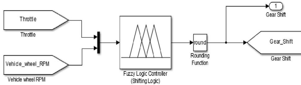
Fig. 5. Shifting Logic Subsystem block
