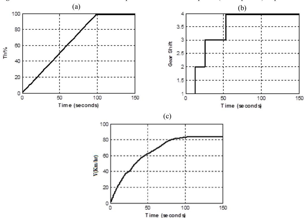
Fig. 8. Simulation results for throttle valve position set at 100% ramp with (1% per sec) slope up to 100 sec then stay constant for 150 sec
