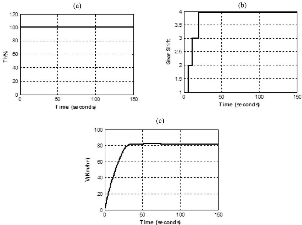
**Fig. 9.** Simulation results for throttle valve position set at 100% at full engine load for 150 sec
