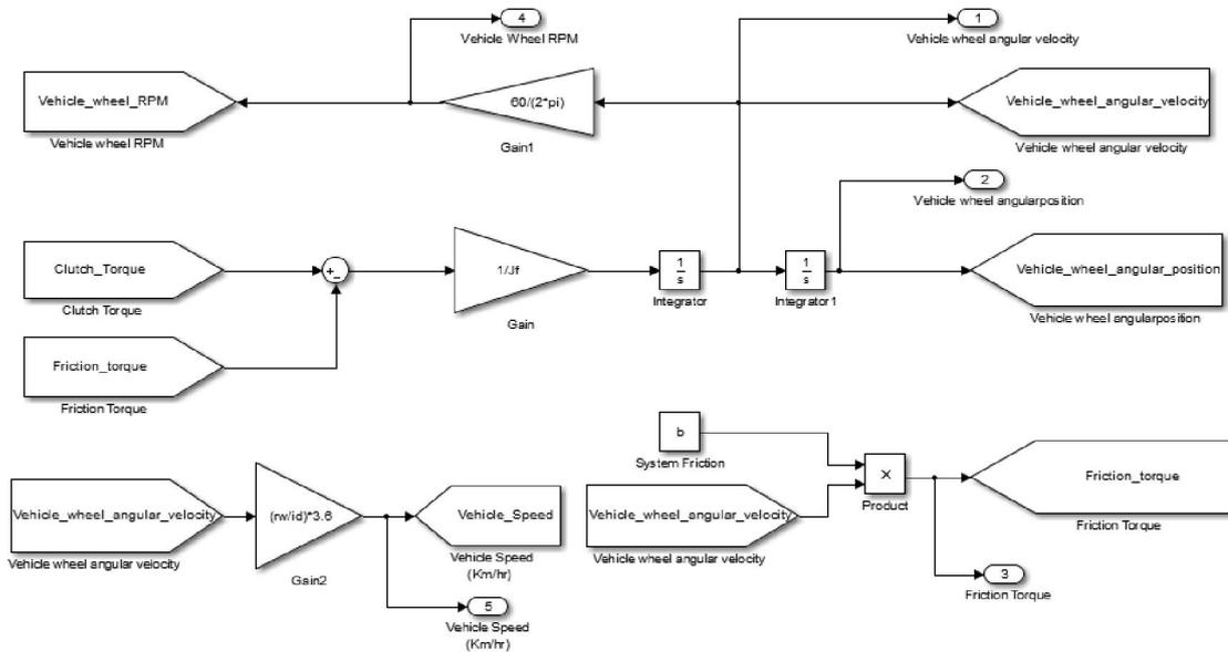
Fig. 4. Vehicle Body Subsystem block
