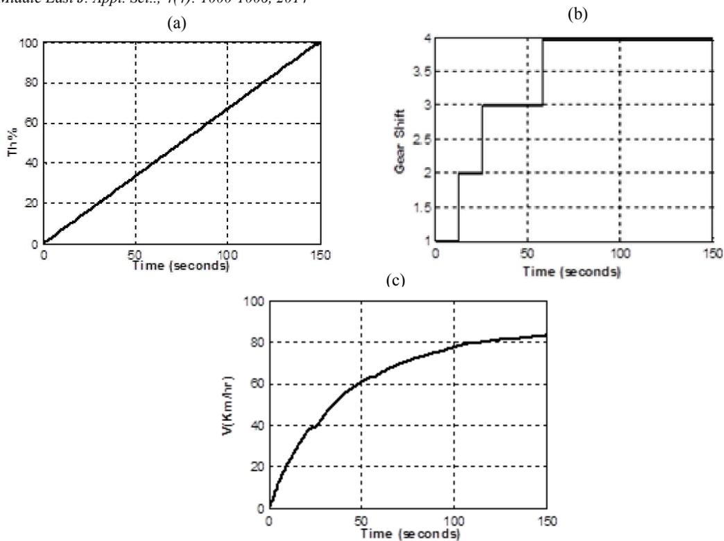
Fig. 7. Simulation results for throttle valve position set at 100% ramp with (0.66% per sec) slope for 150 sec
