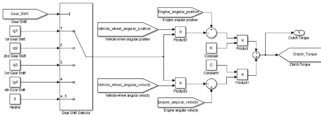
Fig. 3. Clutch and Gearbox Subsystem Block
