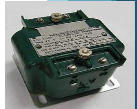
instrument isolation transformer showing two polarity marking conventions
