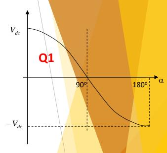
Changing the firing angle of the single phase thyristor converter will change the magnitude of  $V_a$  by changing the firing angle, keeping the same direction of current. Thus motor will operate in Q1 and Q4
