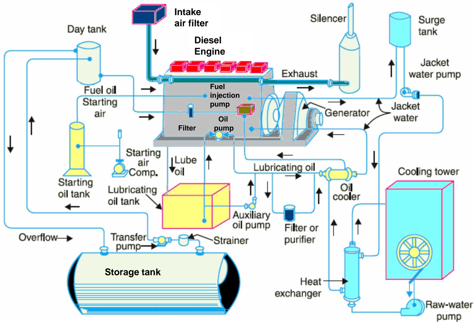
**Schematic arrangement of Diesel Power Plant**
