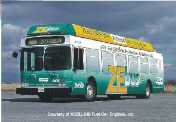
Phase 4 Bus (2000). This bus endured desert conditions during a 1 year field trial in Palm Springs.
