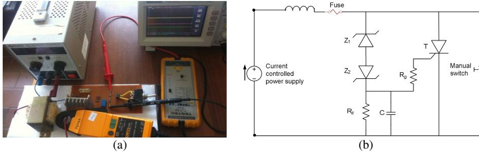
Fig. 5: Test circuit experimental set-up
