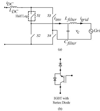
Fig. 1: Single phase grid connected CSI
