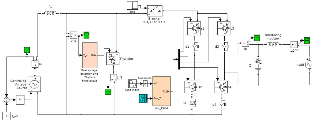
Fig. 3: Proposed system model using MATLAB/SIMULINK
