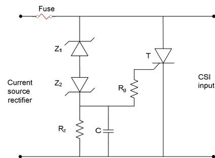
Fig. 2: Proposed over-voltage protection circuit
