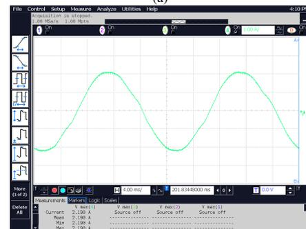
Fig. 11: Grid current experimental results
