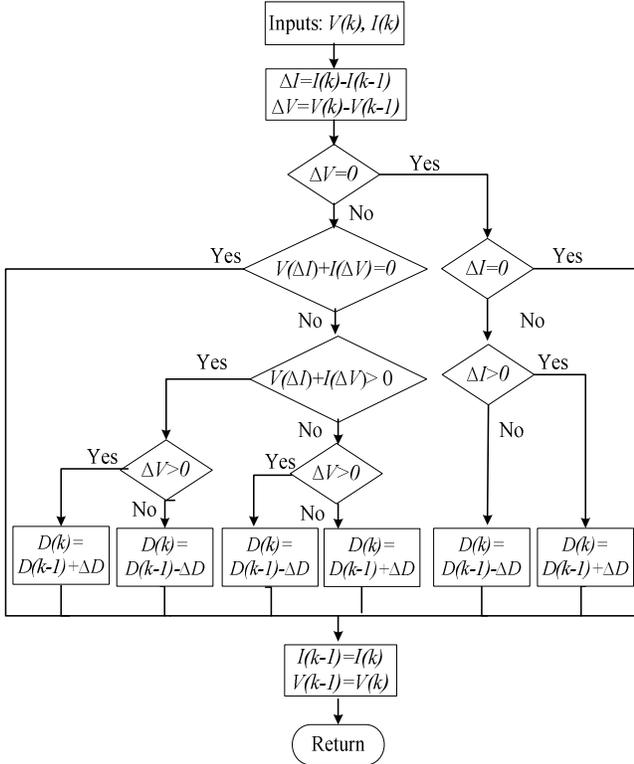
Fig. 6: Flowchart of the proposed modified Inc.Cond. algorithm
