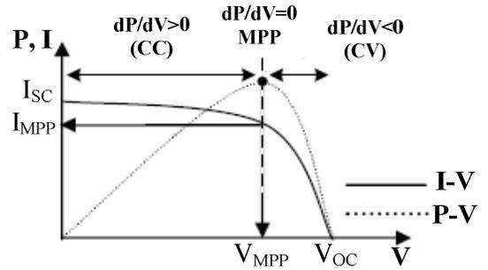
Fig. 3: PV array  $I-V$  and  $P-V$  characteristics
