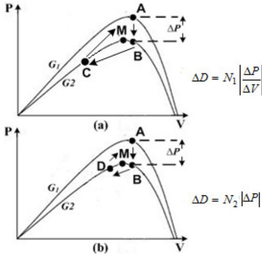
Fig. 7: MPPT algorithm performance, under irradiance change, when adopting (a)  $\Delta P/\Delta V$  based variable step, (b) proposed  $\Delta P$  based variable step
