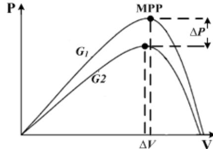
Fig. 4: PV array  $P-V$  characteristics under two different irradiance levels
