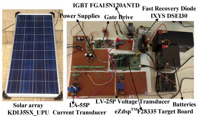
Fig. 12: Test rig photograph
