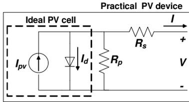
Fig. 2: PV cell single diode model
