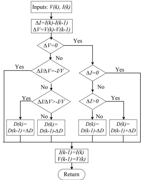
Fig. 5: Flowchart of conventional Inc.Cond. algorithm
