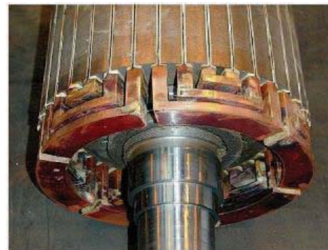
Figure 9. Nested loop rotor 4 pole – 8 pole (4/8) BDFM
