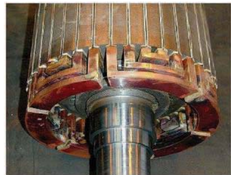
Figure 9. Nested loop rotor 4 pole – 8 pole (4/8) BDFM
