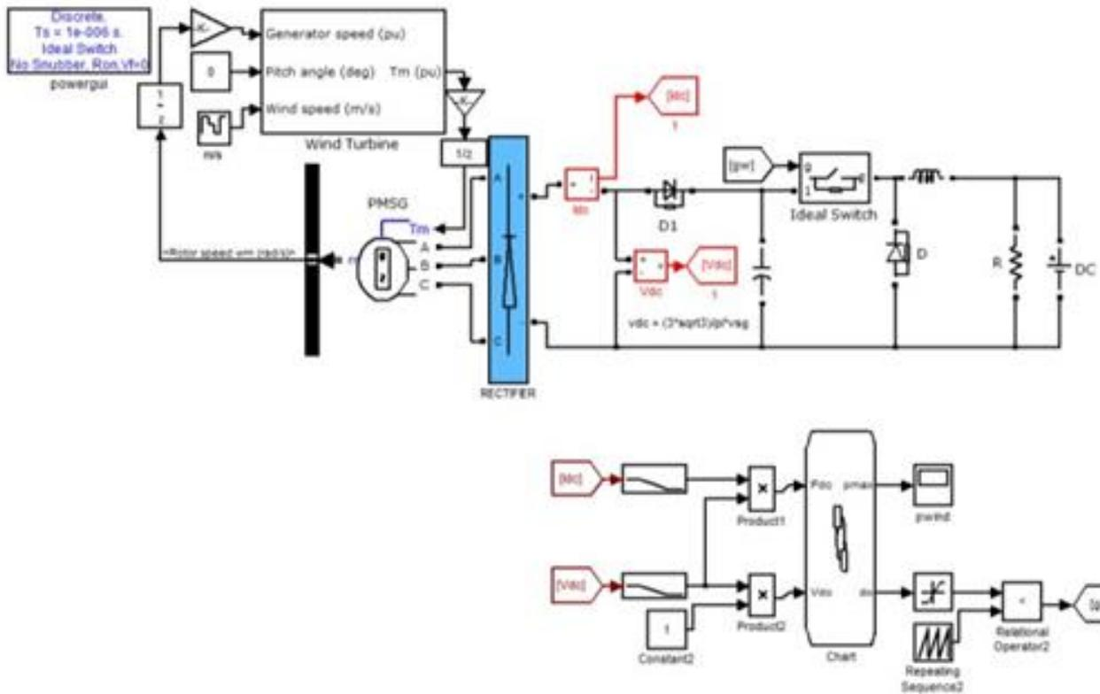
Figure 6: WECS utilizing the proposed State-Flow based MPPT technique MATLAB/SIMULINK<sup>®</sup> simulation diagram
