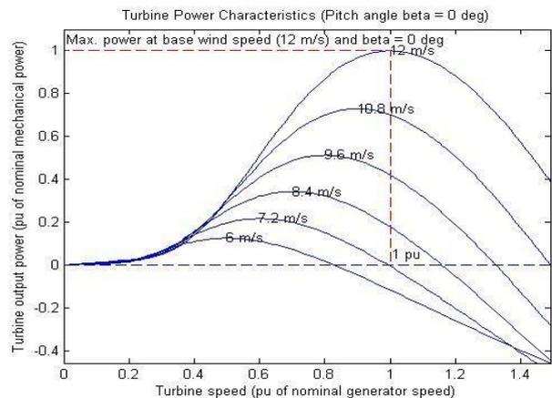
Figure 7: Simulated PMSG characteristics
