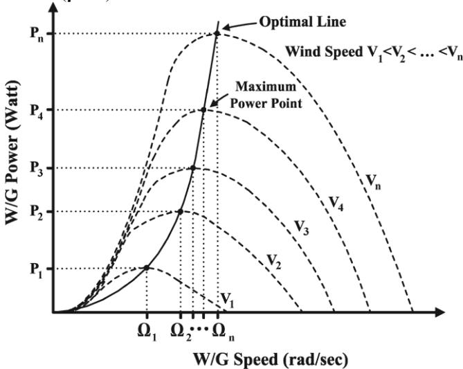
Figure 2: PMSG power curves at various wind speeds.
