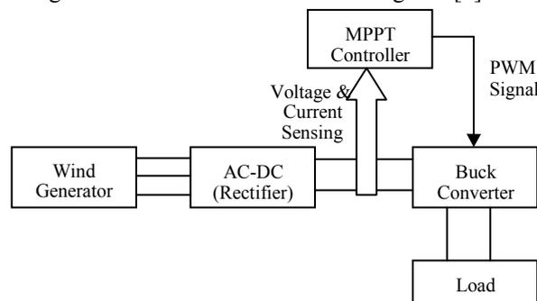
Figure 1: Wind energy conversion system block diagram
