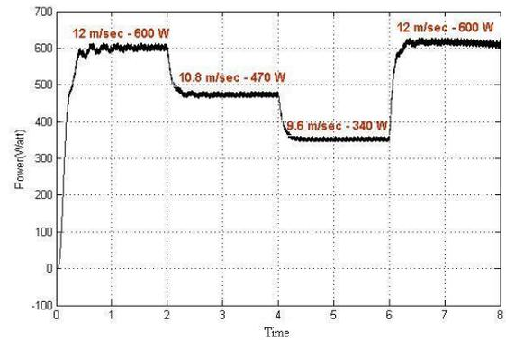
Figure 10: Simulation for 4 different speeds
