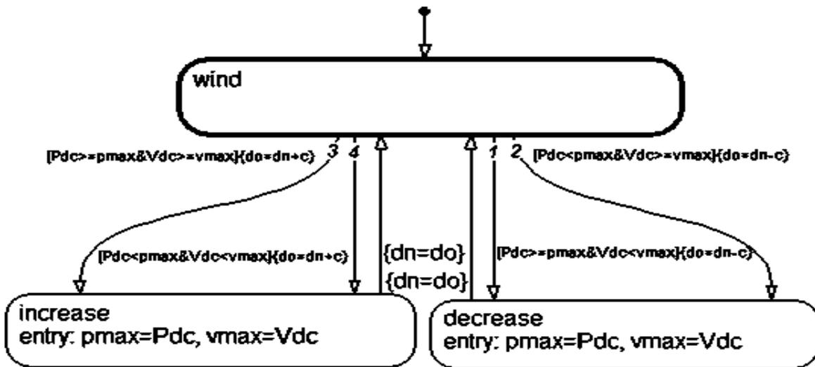
Figure 5: Proposed State-Flow based Wind MPPT technique
