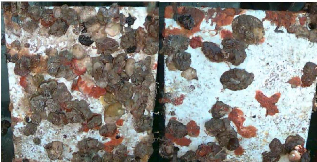
Fig. 9: Photographs of panels exposed at U. of Hawaii fouled with hard and soft fouling organisms [K. Truby et al, 2000]
