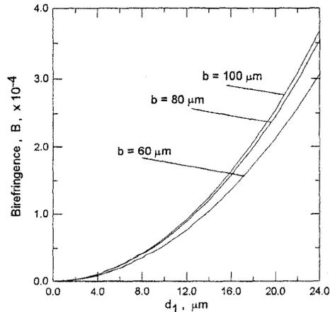
Fig. (4) The dependence of the material birefringence, in a panda fiber, on  $d_1$ , the radius of the SAZ, at different cladding radius,  $b$ , values.
