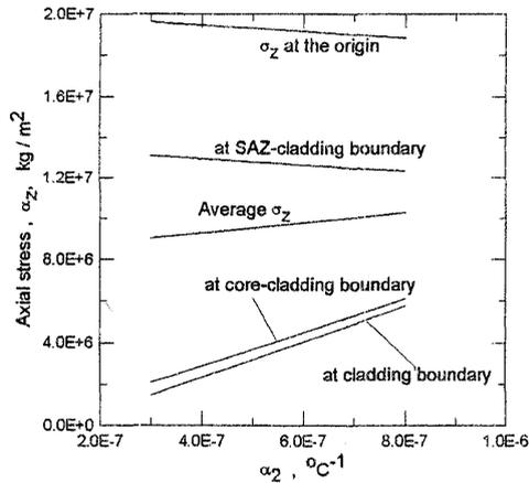
Fig. (5) The axial stress component,  $\sigma_z$ , at certain points, of the panda fiber, as a function of the thermal expansion coefficient of the cladding material.
