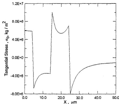
Fig. (8) Tangential stress,  $\sigma_\theta$ , along x-axis in a bow-tie fiber.
