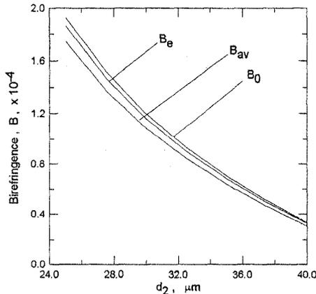
Fig. (3) The different representations of the material birefringence, in a panda fiber, as a function of  $d_2$ , the distance from the origin to the SAZ center.
