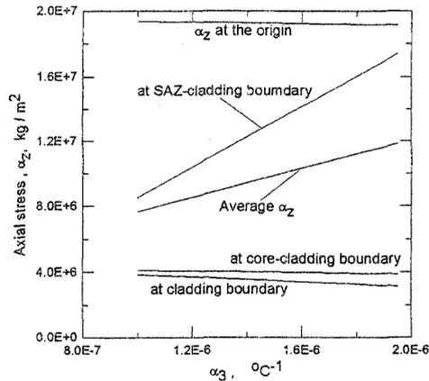
Fig. (6) The axial stress component,  $\sigma_z$ , at certain points, of the panda fiber, as a function of the thermal expansion coefficient of the SAZ material.
