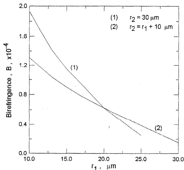
Fig. (9) Variation of the average birefringence,  $B$ , with respect to  $r_1$ , the inner radius of the SAZ, in a bow-tie fiber.
