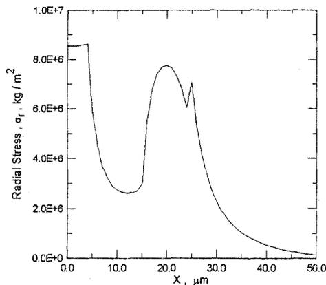
Fig. (7) Radial stress,  $\sigma_r$ , along x-axis in a bow-tie fiber.
