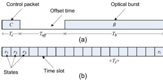
Fig. 1. (a) Transmission of an optical burst (b) slotted timing diagram.
