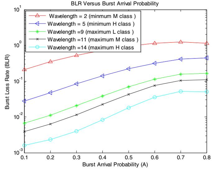
Fig.3. Burst arrival probability ( $A$ ) versus BLR of three classes with  $\rho=0$ ,  $\ell=100$  and  $w < \ell$
