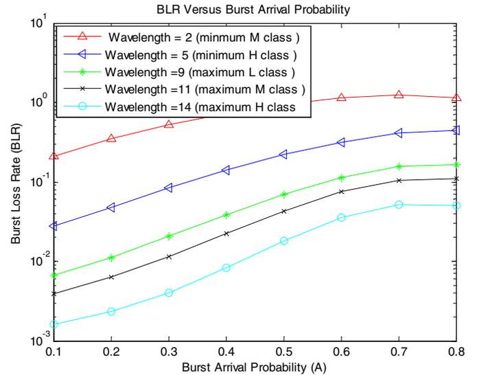
Fig.4. Burst arrival probability ( $A$ ) versus BLR of three classes with  $\rho=1$ ,  $\ell=100$  and  $w < \ell$
