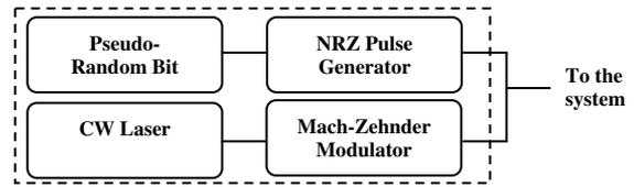
Fig. 5. Optical transmitter.
