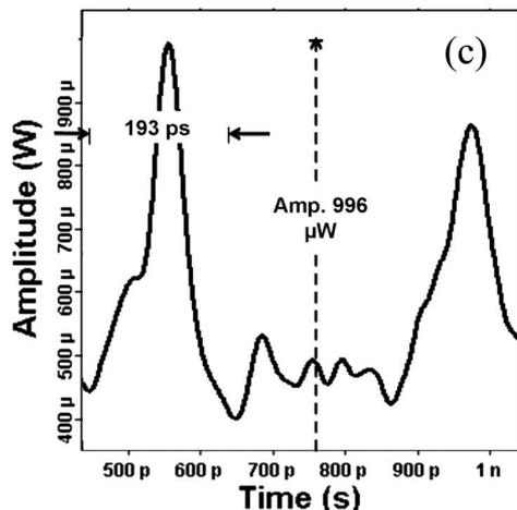
Fig. 8. Performance of (a) linearly chirped AFBG, (b) square-chirped AFBG, and (c) cubic-chirped AFBG as a dispersion compensation unit (point 3, Fig. 4, after optical amplifier).
