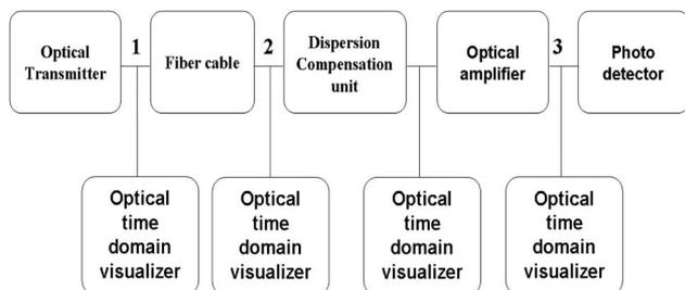
Fig. 4. Proposed system used to evaluate different dispersion compensation techniques.
