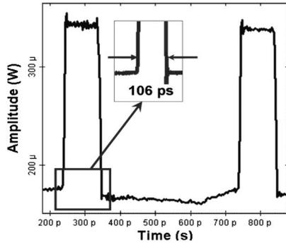
Fig. 11. Signal after amplifier and optimum DCF length merged with linearly chirped tanh FBG for dispersion compensation (point 3, Fig. 4, after optical amplifier).
