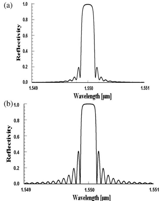
Fig. 3. (a) Normalized reflectivity spectrum of tanh CFBG and (b) normalized reflectivity spectrum of uniform CFBG.
