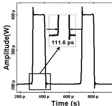
Fig. 9. Signal after DCF (point 3, Fig. 4, after optical amplifier).
