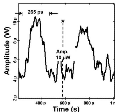
Fig. 7. Signal after 100 km of SMF (point 2, Fig. 4).
