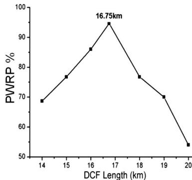
Fig. 12. PWRP as a function of DCF length for a combination of DCF with linearly chirped AFBG.
