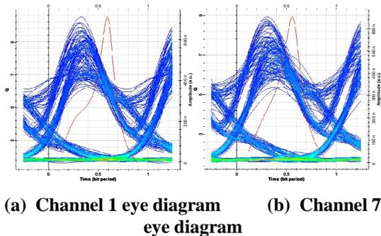
**Figure 8.** Eye diagrams for random channels 1 and 7 at 5 Gbit/s over 60 km. BER
