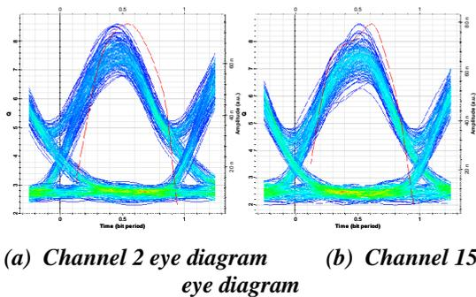
**Figure 7.** Eye diagrams for random channels 2 and 15 at 1 Gbit/s over 80 km. BER
