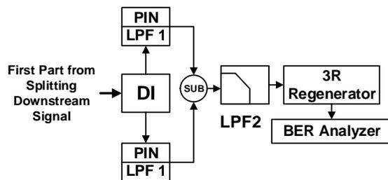
Figure 3. DPSK Receiver in each ONU.
