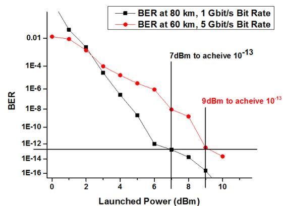
**Figure 6. Optical Launched power (dBm) versus BER**
