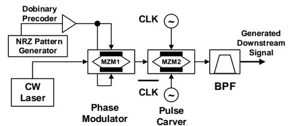
Figure 2. The optical RZ-DPSK transmitter
