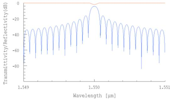
Fig. 4. Transmittivity/Reflectivity (dB) vs Wavelength ( $\mu\text{m}$ ) for uniform FBG ( $L=10000 \mu\text{m}$  and  $\Delta n_{ac}=4 \times 10^{-4}$ )
