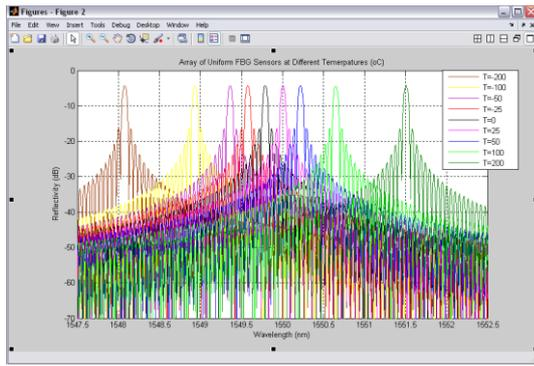
Fig. 11. Array of Uniform FBG sensors at different Temperatures ( $^{\circ}\text{C}$ ) Ranging from  $-200$  to  $200^{\circ}\text{C}$  and at constant  $L = 10000 \mu\text{m}$  and  $\Delta n_{ac} = 4 \times 10^{-4}$
