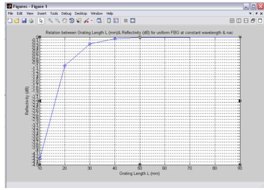
Fig. 6. Grating Length L (mm) vs Reflectivity (dB) at constant wavelength  $\lambda = 1550 \text{ nm}$  and  $\Delta n_{ac}=4 \times 10^{-4}$
