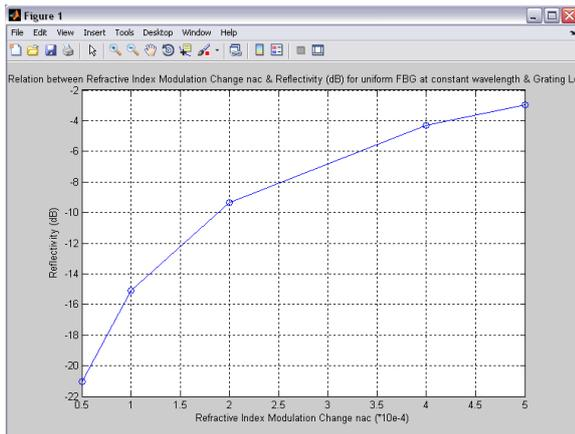
Fig. 8. Refractive index Modulation change ( $\Delta n_{ac}$ ) vs Reflectivity (dB) at constant wavelength  $\lambda = 1550$  nm and  $L=10$  mm
