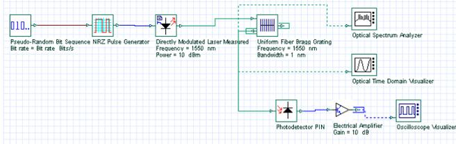
Fig. 3. Block Diagram of Temperature Sensor System setup using uniform FBG
