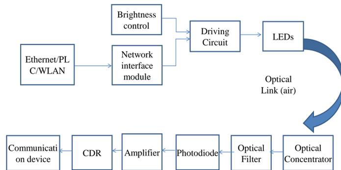
Fig.1 VLC communication System Block diagram
