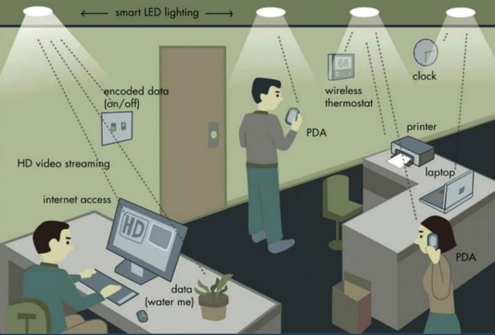
Fig.5: VLC system application
