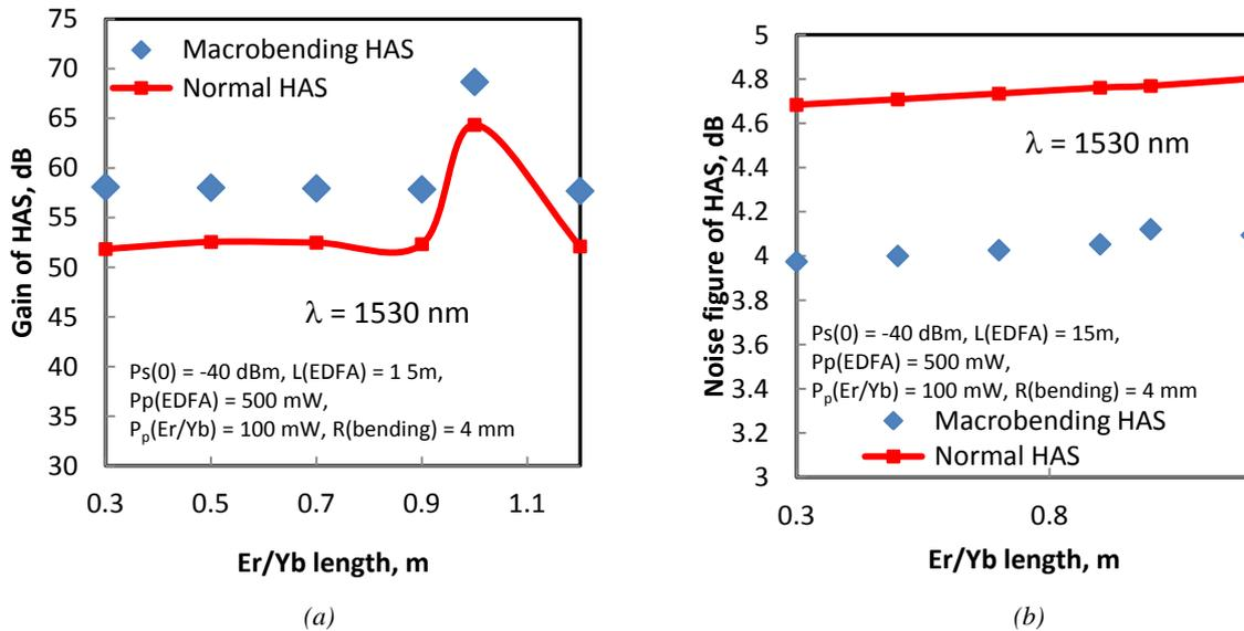
Fig.8. HAS (a) gain and (b) noise figure as functions of Er/Yb co-doped length for bent and normal cases.
