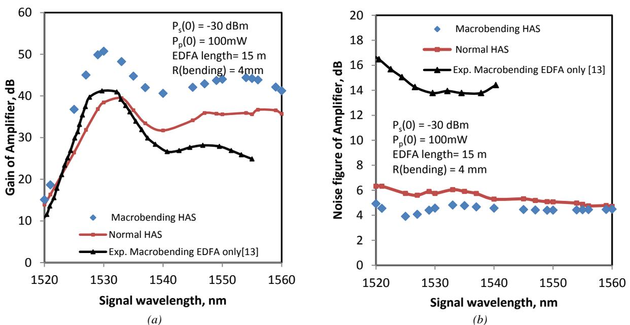
Fig.9. HAS performance comparison (a) gain and (b) noise figure as functions of signal wavelength for macrobending EDFA only [13] with our macrobent and normal cases.
