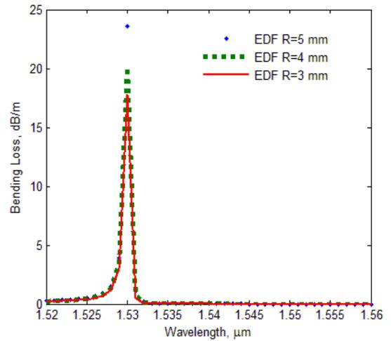
Fig.2 EDF bending-loss coefficient against wavelength for different bending radii 3, 4 and 5 mm.
