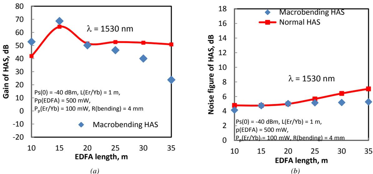
Fig.7 HAS (a) gain and (b) noise figure as function of EDFA length for bent and normal cases.
