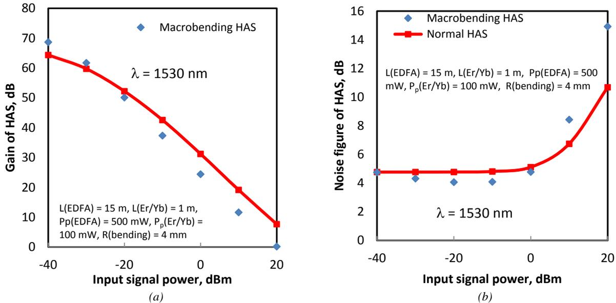
Fig.6. HAS (a) gain and (b) noise figure as function of input signal power for bent and normal cases.
