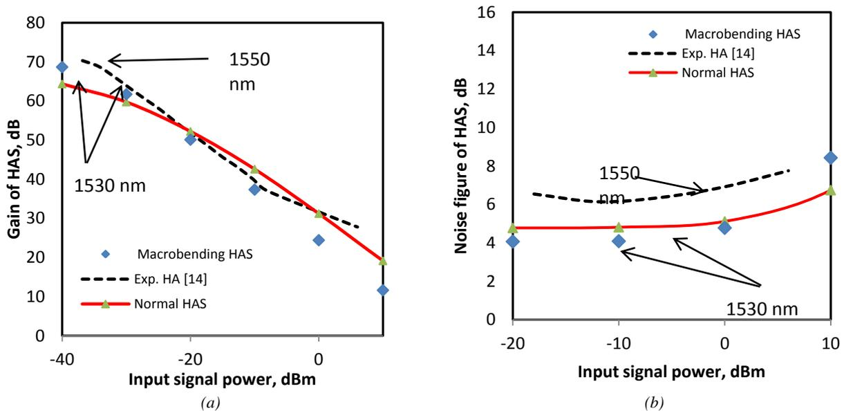
Fig.10. HAS performance comparison (a) gain and (b) noise figure as functions of input signal power for hybrid amplifier [14] with our macrobent and normal cases.
