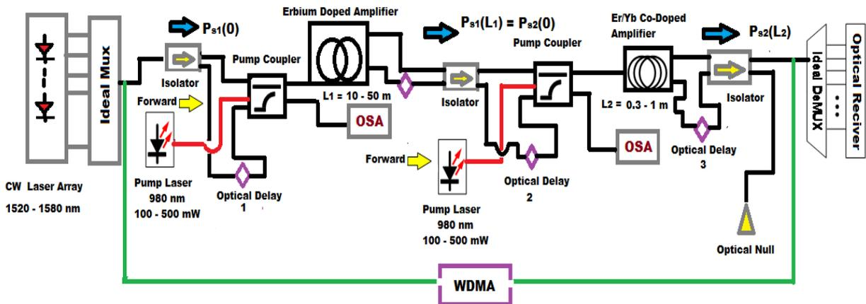
Fig.1. Hybrid macrobent EDFA/EYCDFA experimental set-up.
