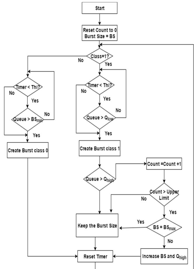
Fig.3 Flow diagram for adaptive burst assembly.
