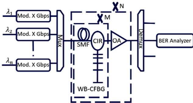
Fig. 2. WBDC CFBG system structure, CIR is a circulator.
