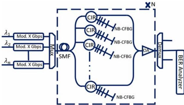
Fig. 3. Multi-narrow CFBG system structure.
