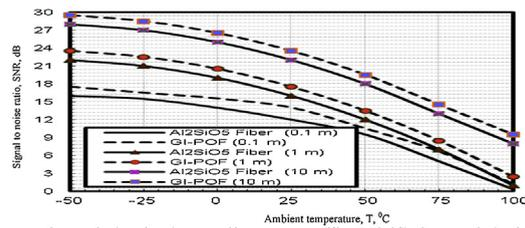
**Fig. 3.** Signal to noise ratio versus ambient temperature at different optical fiber interconnection lengths.
