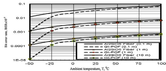
**Fig. 4.** Bit error rate versus ambient temperature at different optical fiber interconnection lengths.
