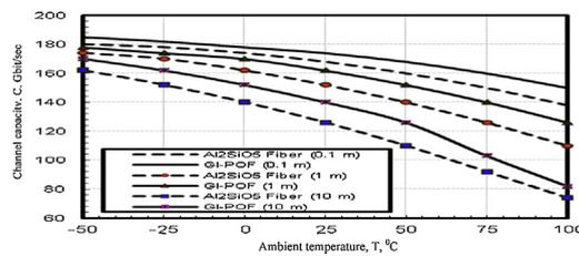
**Fig. 2.** Channel capacity versus ambient temperature at different optical fiber interconnection lengths.
