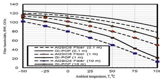
**Fig. 1.** Fiber bandwidth versus to ambient temperature at different optical fiber interconnection lengths.
