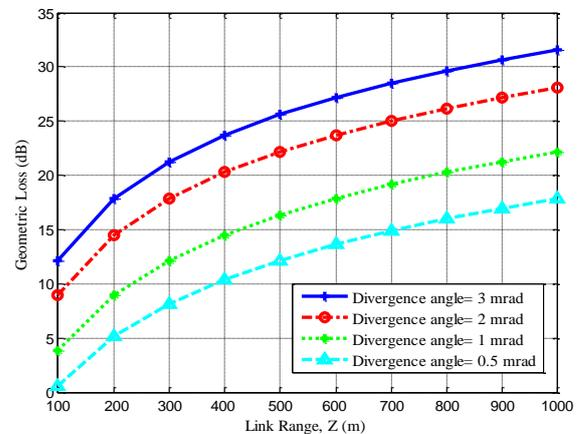
Fig. 2. Geometric loss vs. link length
