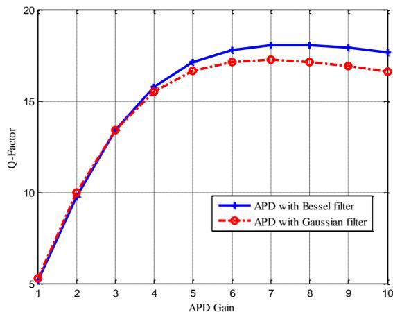
Fig. 7. The Q-factor vs. APD gain for SISO over log-normal channel with Bessel and Gaussian filters for 500 m link range
