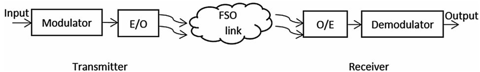
Fig. 1. Typical schematic diagram of an FSO system.
