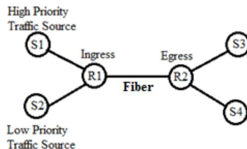
Fig. 4. Optical network topology
