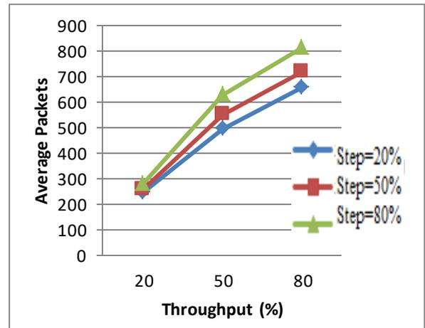
Fig. 11. Average number of packets per burst for high priority traffic at with 50 ms threshold
