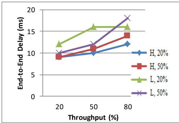
Fig. 12. Delay for high (H) and low (L) priority traffic with 20 ms threshold
