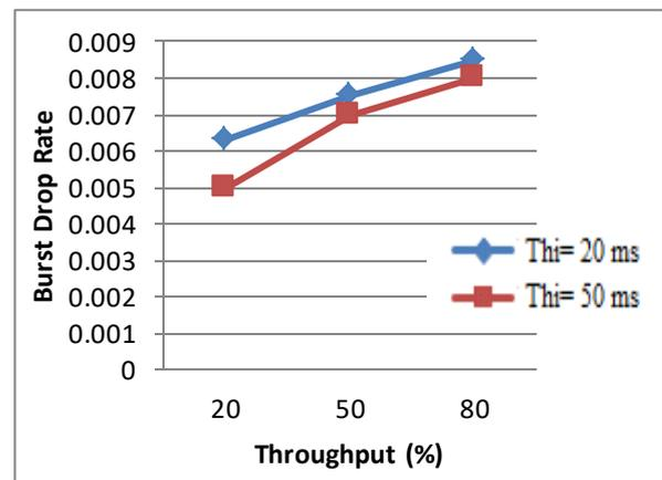
Fig. 9. Burst drop rate for high priority traffic with 80% adaptation step size
