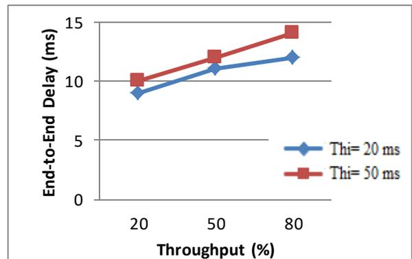
Fig. 15. Delay for high priority traffic with 50% adaptation step size
