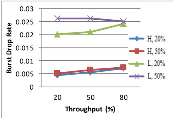
Fig. 6. Burst drop rate for high (H) and low (L) priority traffics at 50 ms threshold
