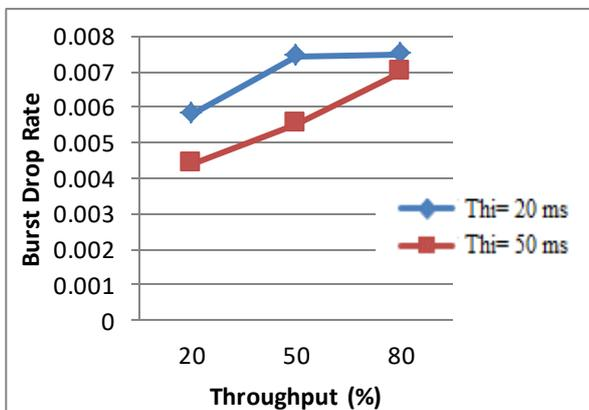
Fig. 7. Burst drop rate for high priority traffic with 20% adaptation step size
