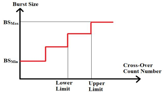
Fig. 2. Discrete type burst size decision technique
