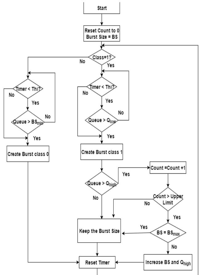
Fig. 3. Flow diagram for smart burst assembly
