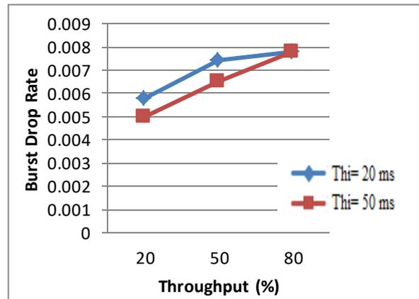
Fig. 8. Burst drop rate for high priority traffic with 50% adaptation step size
