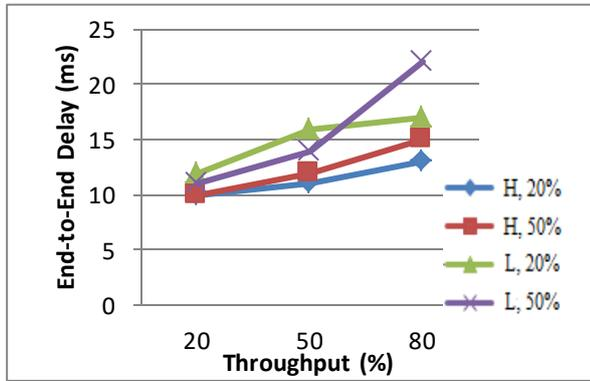
Fig. 13. Delay for high (H) and low (L) priority traffic with 50 ms threshold
