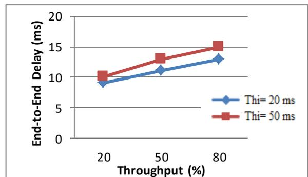
Fig. 16. Delay for high priority traffic with 80% adaptation step size
