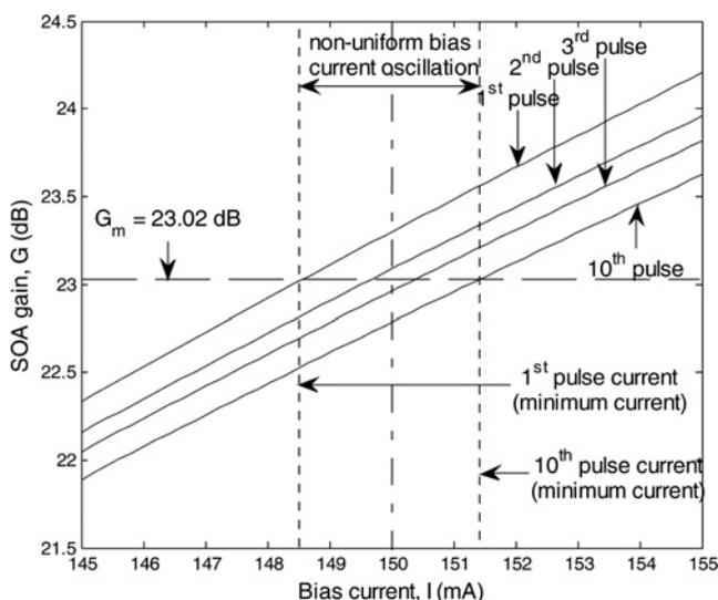
**Fig. 3** SOA gain response of all pulses within the packet to the uniform bias current
