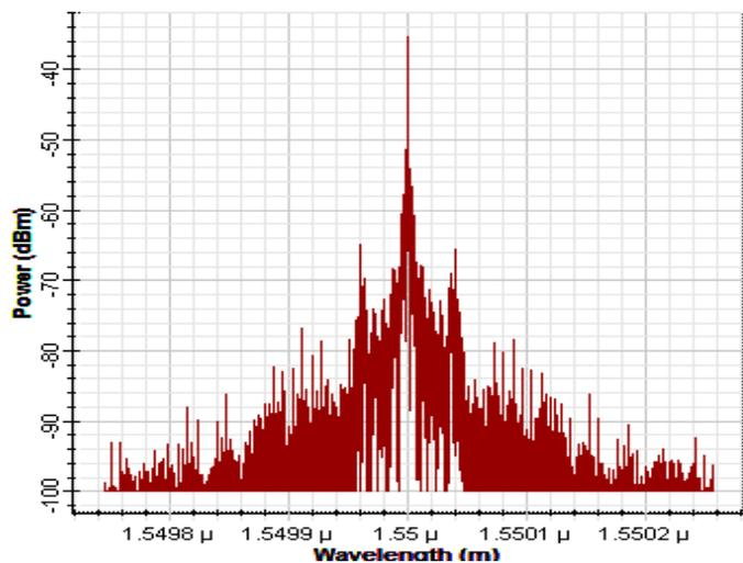
Fig.3 Signal power at receiver for moderate fog weather condition at the maximum pointing error calculated at Table 3
