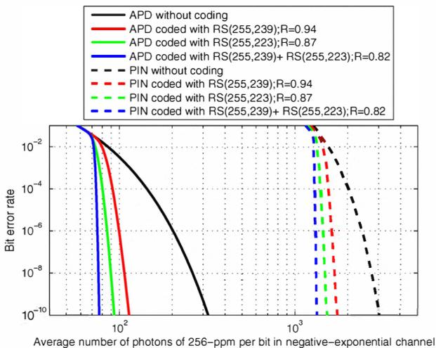
Figure 3. BER for 256-PPM using PIN/APD receivers in negative-exponential channel.
