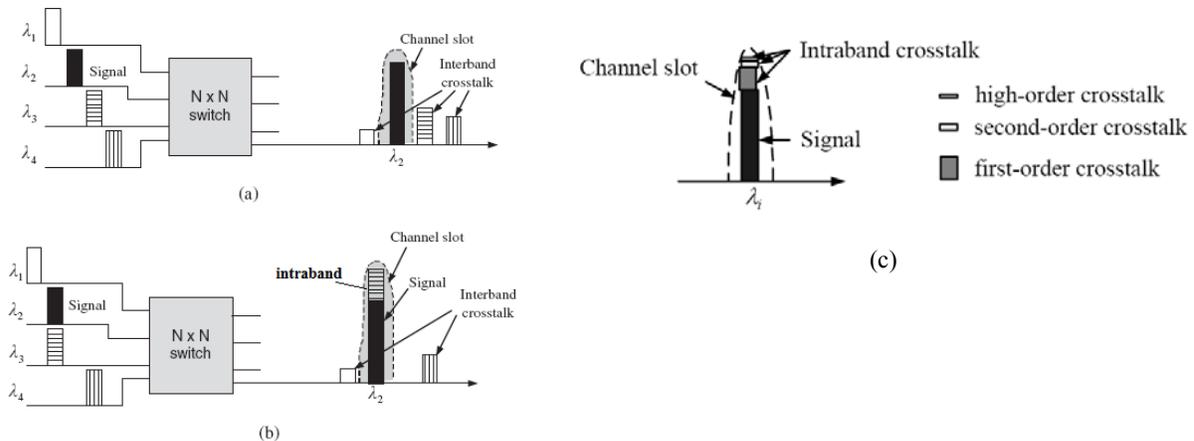
Fig. 1 Switched induced crosstalk: (a) interband, and (b,c) intraband.
