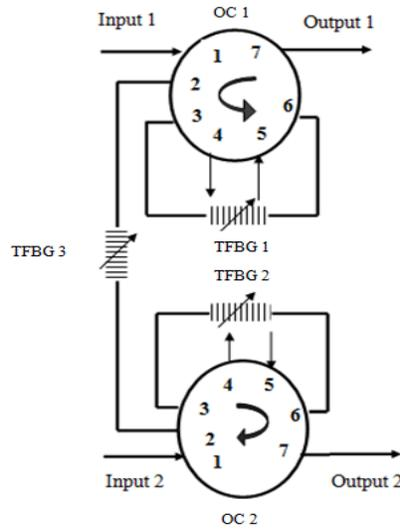
Fig. 3  $2 \times 2$  OXADM using MOC and TFBGs.
