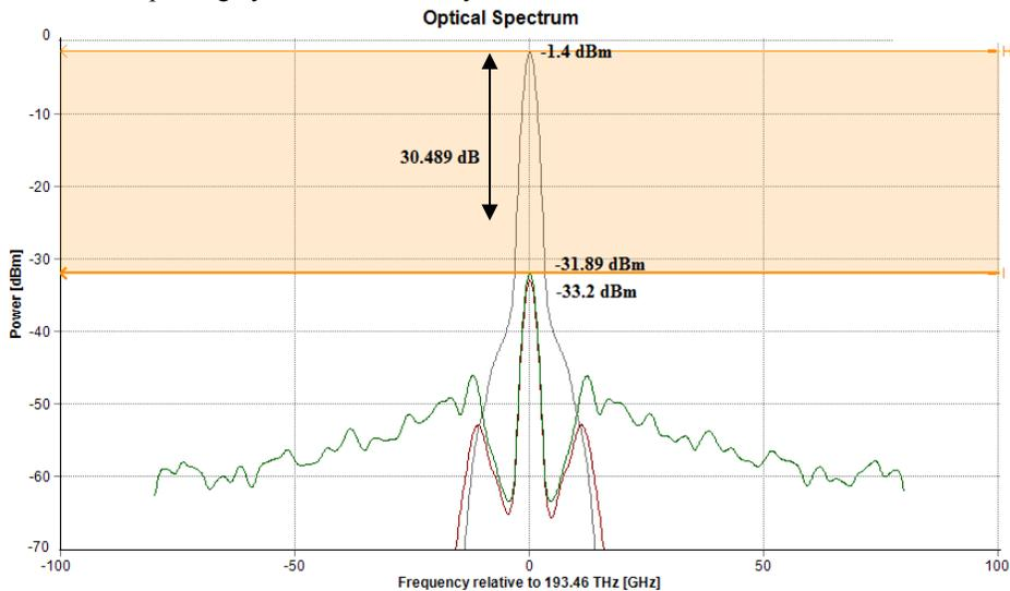
Fig. 5 Drop signal from port 4 at OC1 for OXADM1.
