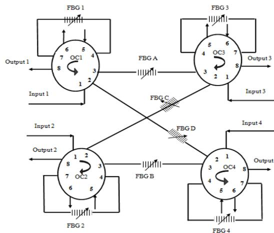
Fig. 8 Proposed architecture of bi-directional OXADM.
