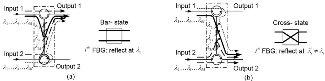
Fig. 2 Two switching states of a  $2 \times 2$  OXC (a) bar-state and (b) cross-state.
