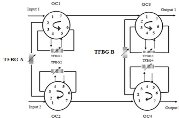
Fig. 7 Multistage structure 2×2 OXADM.
