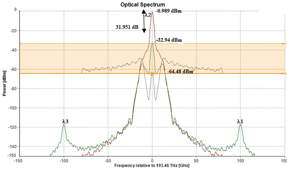
Fig. 4 Output 1 from OC1 when TFBG3 tuned at 193.46 THz for OXADM1.
