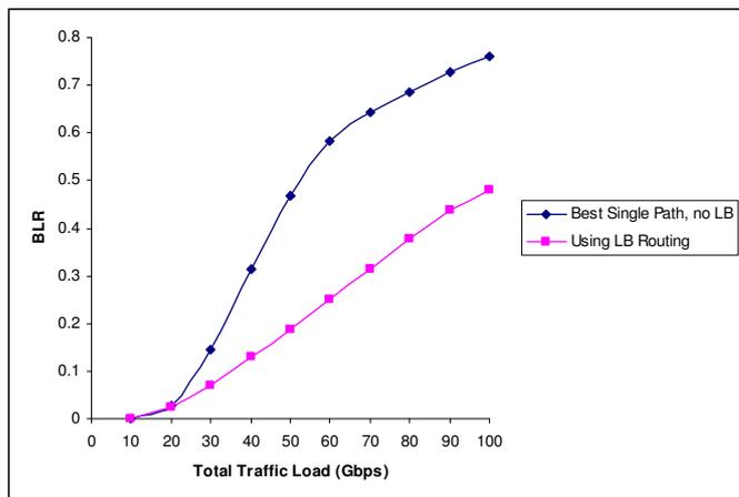
Figure 11 Relation between total traffic load and BLR before and after using load balance routing.
