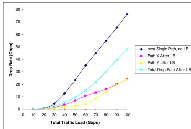
Figure 10 Relation between total traffic load and drop rate before and after using load balance routing.
