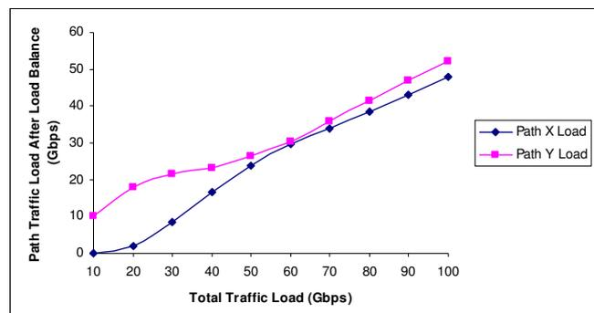
Figure 8 Relation between total traffic load and its distribution on different paths after using unequal load balance routing.
