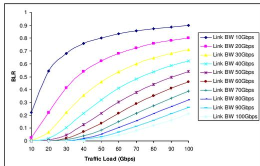
Fig. 5 Relation between BLR and traffic load at different link bandwidths, at n = 10.
