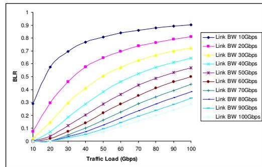
Fig. 4 Relation between BLR and traffic load at different link bandwidths, at n = 5.
