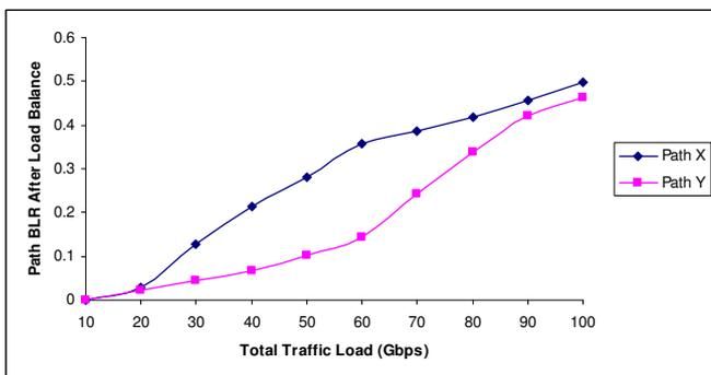
Figure 9 Relation between total traffic load and path BLR after using unequal load balance routing.
