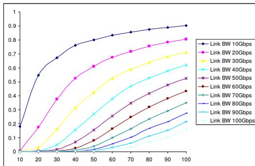
Fig. 6 Relation between BLR and traffic load at different link bandwidths, at n = 20.
