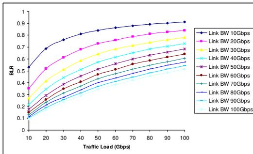
Fig. 3 Relation between BLR and traffic load at different link bandwidths, at n = 1.
