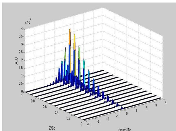
Figure 12 The evolution for RZ-train of solitons of width 0.5 ps, down an EDFA of length 12.5 m, doping level  $40 \times 10^{23}$  atoms/m<sup>3</sup>, and  $\beta_2 = -20 \times 10^{-27}$  s<sup>2</sup>.m<sup>-1</sup> at  $\lambda = 1.55$   $\mu$ m. The time slot between the pulses = 7 ps (frequency domain).
