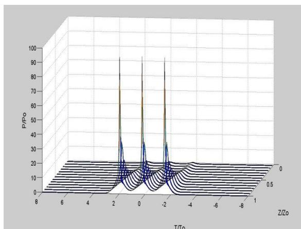
Figure 11 The evolution for RZ-train of solitons of width 0.5 ps, down an EDFA of length 12.5 m, doping level  $40 \times 10^{23}$  atoms/m<sup>3</sup>, and  $\beta_2 = -20 \times 10^{-27}$  s<sup>2</sup>.m<sup>-1</sup> at  $\lambda = 1.55$   $\mu$ m. The time slot between the pulses = 7 ps (time domain-back view).
