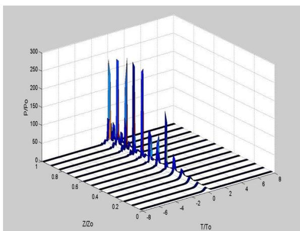
Figure 14 The evolution for RZ-train of solitons of width 0.5, down an EDFA of length 12.5 m, doping level  $40 \times 10^{23}$  atoms/m<sup>3</sup>, and  $\beta_2 = -20 \times 10^{-27}$  s<sup>2</sup>.m<sup>-1</sup> at  $\lambda = 1.55$   $\mu$ m. The time slot between the pulses = 0.5 ps (frequency domain).
