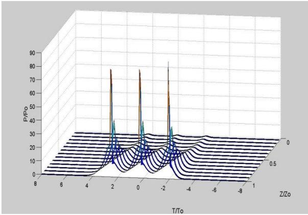
Figure 3 The evolution for RZ-train of solitons of width 0.2 ps down an EDFA of length 2 m, doping level  $50 \times 10^{23}$  atoms/m<sup>3</sup>, and  $\beta_2 = -20 \times 10^{-27}$  s<sup>2</sup>.m<sup>-1</sup> at  $\lambda = 1.55$   $\mu$ m. The time slot between the pulses = 9 ps (time domain -back view).
