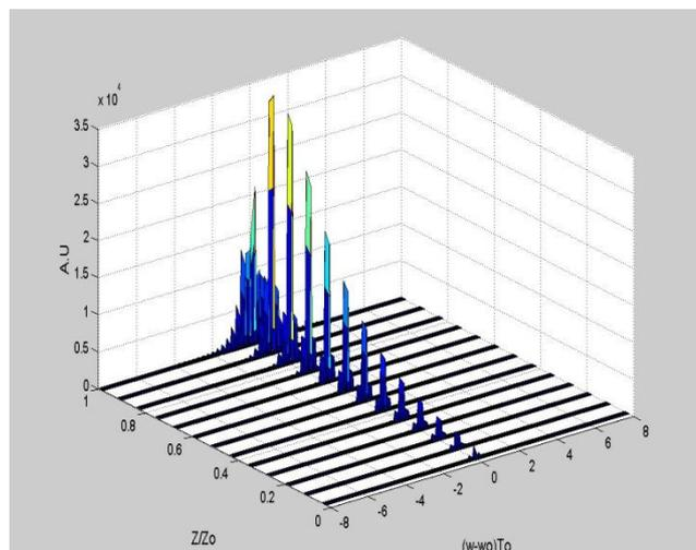
Figure 10 The evolution for RZ-train of solitons of width 0.5 ps down an EDFA of length 12.5 m, doping level  $40 \times 10^{23}$  atoms/m<sup>3</sup>, and  $\beta_2 = -20 \times 10^{-27}$  s<sup>2</sup>.m<sup>-1</sup> at  $\lambda = 1.55$   $\mu$ m. The time slot between the pulses = 8 ps and bit rate = 125 Gbps (frequency domain).
