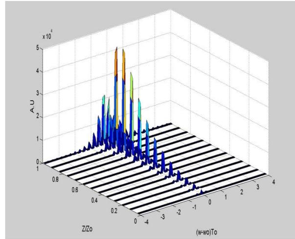
Figure 8 The evolution for RZ-train of solitons of width 0.3 ps, down an EDFA of length 4.5 m, doping level  $45 \times 10^{23}$  atoms/m<sup>3</sup>, and  $\beta_2 = -20 \times 10^{-27}$  s<sup>2</sup>.m<sup>-1</sup> at  $\lambda = 1.55$   $\mu$ m. The time slot between the pulses = 7 ps and the bit rate = 208.3 Gbps (frequency domain).
