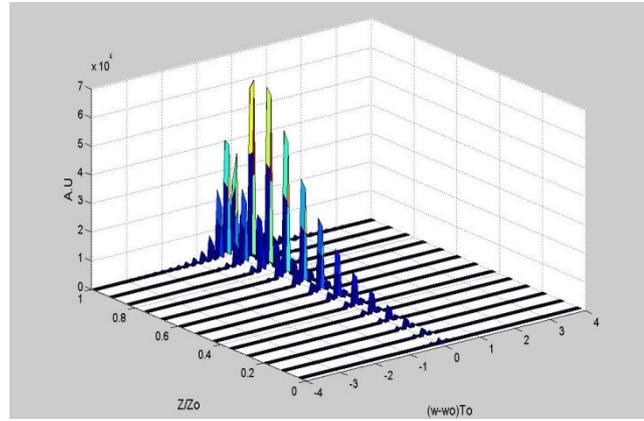
Figure 4 The evolution for RZ-train of solitons of width 0.2 ps down an EDFA of length 2 m, doping level  $50 \times 10^{23}$  atoms/m<sup>3</sup>, and  $\beta_2 = -20 \times 10^{-27}$  s<sup>2</sup>.m<sup>-1</sup> at  $\lambda = 1.55$   $\mu$ m. The time slot between the pulses = 9 ps (frequency domain).
