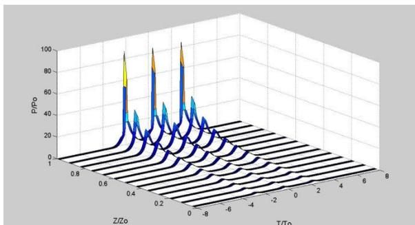
Figure 1 The evolution for RZ-train of solitons of width 0.2 ps down an EDFA of length 2 m, doping level  $50 \times 10^{23}$  atoms/m<sup>3</sup>, and  $\beta_2 = -20 \times 10^{-27}$  s<sup>2</sup>.m<sup>-1</sup> at  $\lambda = 1.55$   $\mu$ m. The time slot between the pulses = 10 ps and the bit rate = 250 Gbps (time domain).
