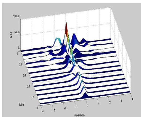
Figure 13 The evolution for RZ-train of solitons of width 0.5, down an EDFA of length 12.5 m, doping level  $40 \times 10^{23}$  atoms/m<sup>3</sup>, and  $\beta_2 = -20 \times 10^{-27}$  s<sup>2</sup>.m<sup>-1</sup> at  $\lambda = 1.55$   $\mu$ m. The time slot between the pulses = 0.5 ps (time domain).
