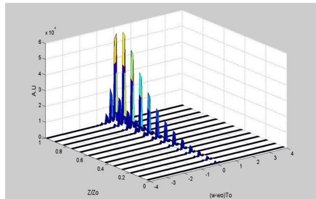
Figure 6 The evolution for RZ-train of solitons of width 0.3 ps down an EDFA of length 4.5 m, doping level  $45 \times 10^{23}$  atoms/m<sup>3</sup>, and  $\beta_2 = -20 \times 10^{-27}$  s<sup>2</sup>.m<sup>-1</sup> at  $\lambda = 1.55$   $\mu$ m. The time slot between the pulses = 8 ps and the bit rate = 208.3 Gbps (frequency domain).
