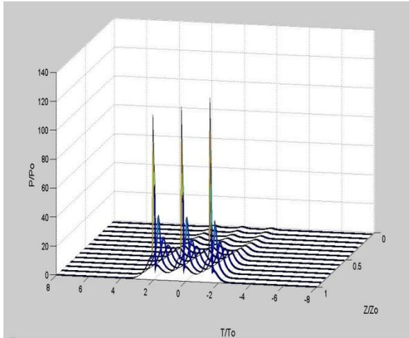
Figure 7 The evolution for RZ-train of solitons of width 0.3 ps, down an EDFA of length 4.5 m, doping level  $45 \times 10^{23}$  atoms/m<sup>3</sup>, and  $\beta_2 = -20 \times 10^{-27}$  s<sup>2</sup>.m<sup>-1</sup> at  $\lambda = 1.55$   $\mu$ m. The time slot between the pulses = 7 ps and the bit rate = 208.3 Gbps (time domain- back view).
