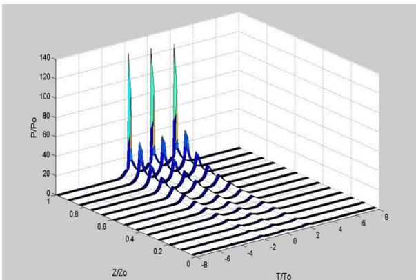
Figure 5 The evolution for RZ-train of solitons of width 0.3 ps down an EDFA of length 4.5 m, doping level  $45 \times 10^{23}$  atoms/m<sup>3</sup>, and  $\beta_2 = -20 \times 10^{-27}$  s<sup>2</sup>.m<sup>-1</sup> at  $\lambda = 1.55$   $\mu$ m. The time slot between the pulses = 8 ps and the bit rate = 208.3 Gbps (time domain).
