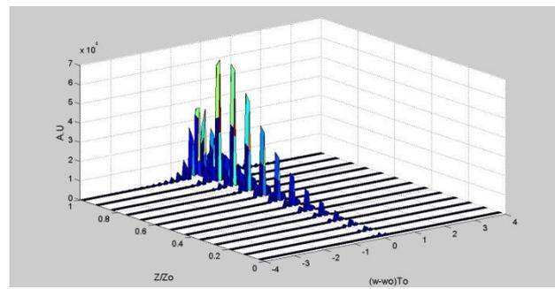
Figure 2 The evolution for RZ-train of solitons of width 0.2 ps down an EDFA of length 2 m, doping level  $50 \times 10^{23}$  atoms/m<sup>3</sup>, and  $\beta_2 = -20 \times 10^{-27}$  s<sup>2</sup>.m<sup>-1</sup> at  $\lambda = 1.55$   $\mu$ m. The time slot between the pulses = 10 ps and the bit rate = 250 Gbps (frequency domain).
