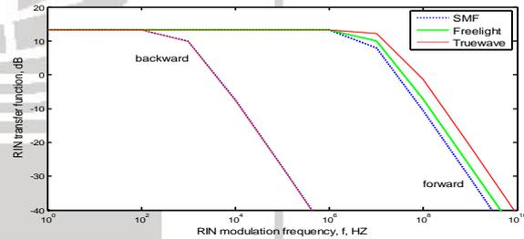
Fig. 9 RIN transfer function  $T^2$ , in the electrical domain, as a function of the RIN modulation frequency. Both forward and backward pumping schemes are considered for a transmission span of 100 km and GR =20 dB.
