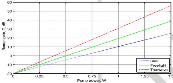
Fig. 2 The Raman gain as a function of pump power for 100 km fiber span of different fiber types.
