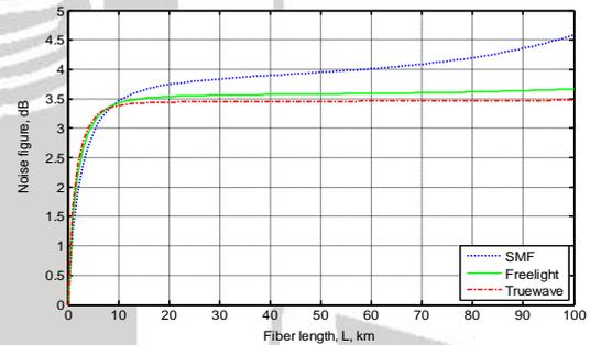
Fig. 5 Noise Figure as a function of fiber length at 800 mW pump power.
