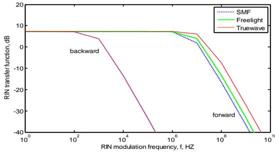
Fig.10 RIN transfer function  $T^2$ , in the electrical domain, as a function of the RIN modulation frequency. Both forward and backward pumping schemes are considered for a transmission span of 100 km and  $GR = 10$  dB.
