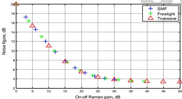
Fig. 8 Noise figure versus on-off Raman Gain for a 100km fiber varying input pump power using different fiber types.
