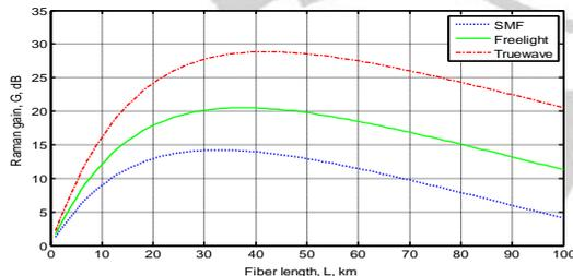
Fig. 3 The Raman net gain as a function of fiber length for different types of fiber at 800 mW pump power.
