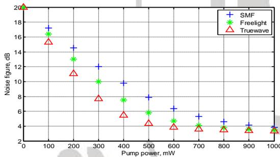
Fig. 7 Noise Figure as a function of pump power for 100 km different fiber types.
