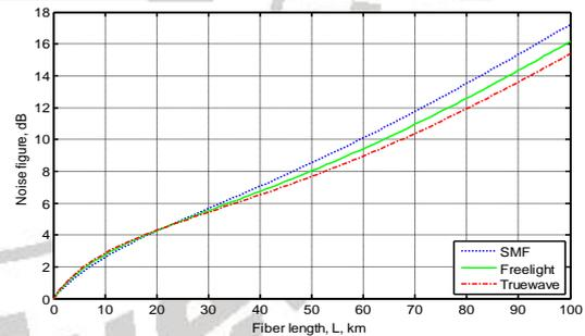
Fig. 6 Noise Figure as a function of fiber length at 100 mW pump power.
