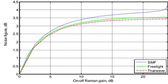
Fig. 4 Noise figure as a function of on-off Raman gain with 800 mw pump power.
