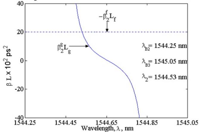
**Fig. 7:** Dispersion compensation design for a channel at 1544.53 nm.
