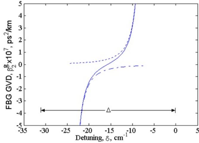
**Fig. 1:** GVD as a function of  $\delta$  for a single grating centered at  $\delta = 0$  (dotted line) and  $\delta = -$  (dot-dashed line), and for two cascaded gratings (solid line).
