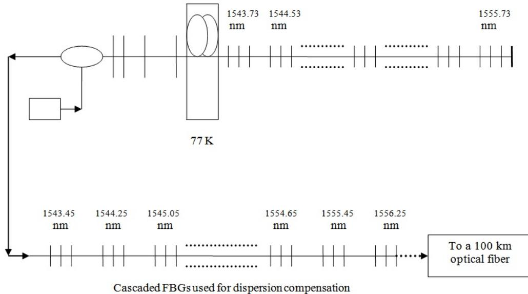
**Fig. 8:** The schematic of 16 channels EDFL followed by the dispersion compensation System.
