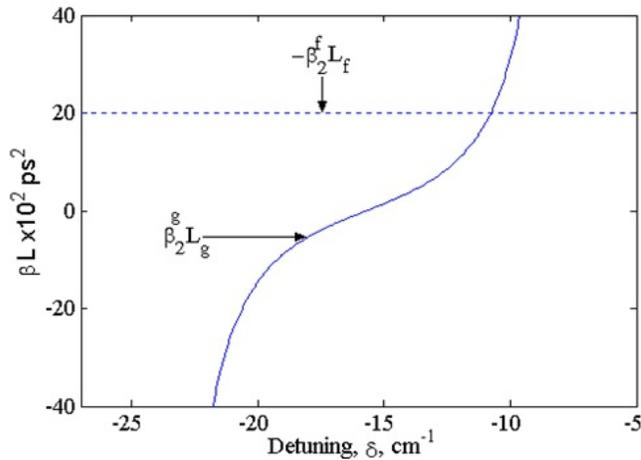
**Fig. 3:** Graphical solution of Eq. (8) for  $L_f = 100 \text{ km}$ ,  $\beta_2^f = -20 \text{ ps}^2/\text{km}$ ,  $k = 7 \text{ cm}^{-1}$ ,  $L_g = 10 \text{ cm}$  and  $\nu = 100 \text{ GHz}$ .
