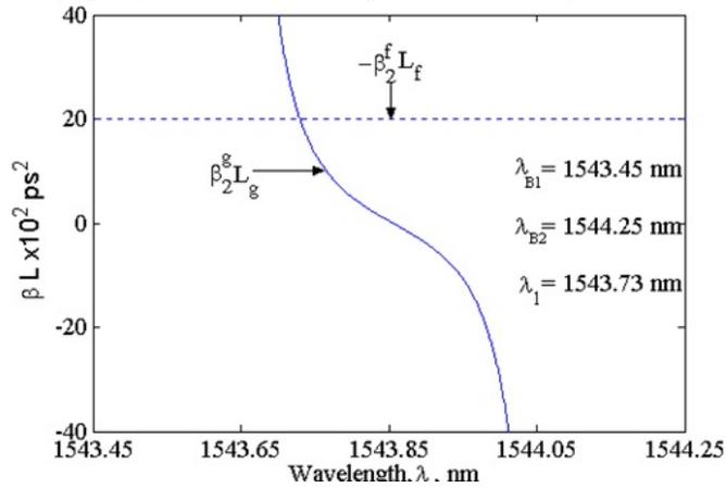
**Fig. 6:** Dispersion compensation design for a channel at 1543.73 nm.
