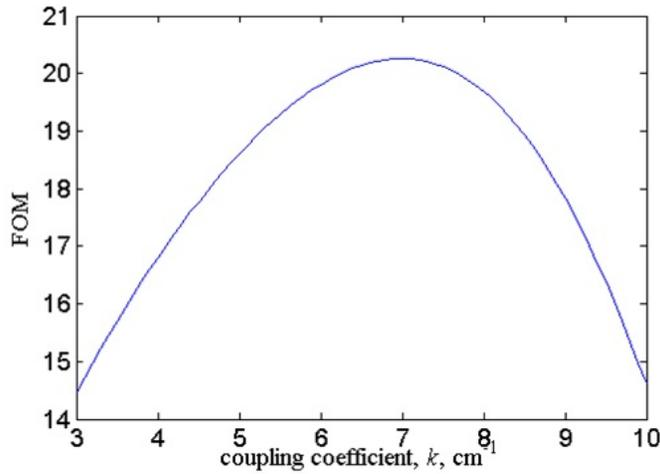
**Fig. 5:** Figure of merit versus coupling coefficient with optimized detuning for each  $k$  for  $\nu = 100$  Ghz.
