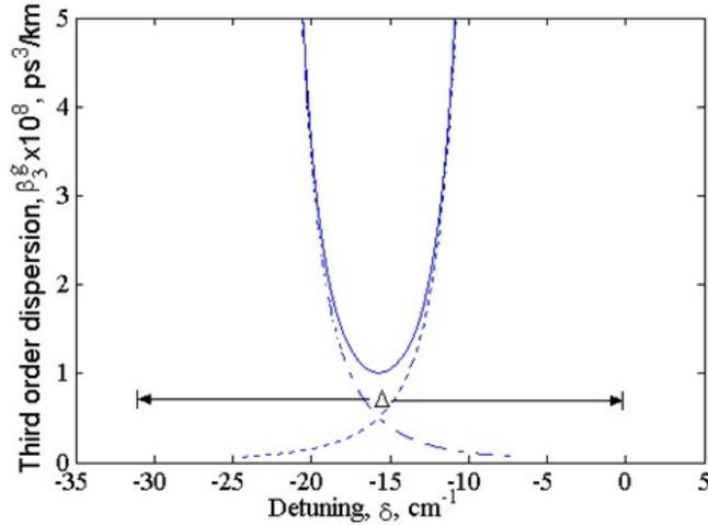
**Fig. 2:** Third order dispersion as a function of  $\delta$  for a single grating centered at  $\delta = 0$  (dotted line) and  $\delta = -$  (dot-dashed line), and for two cascaded gratings (solid line).
