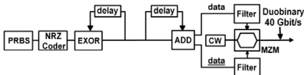
Figure 12 Duobinary transmitter.
