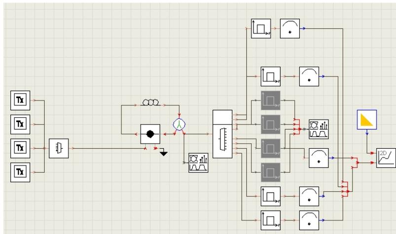
Figure 1 Block diagram of the VPI software for a WDM transmission system.
