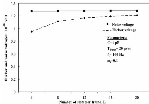
Fig.6 Effect of number of slots per frame for incandescent lighting.
