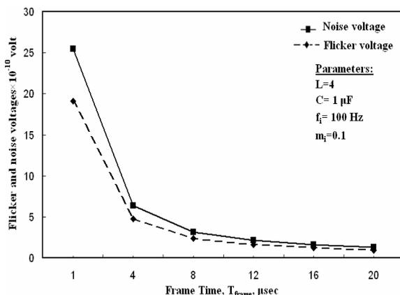
Fig.5 Effect of frame time for incandescent lighting.
