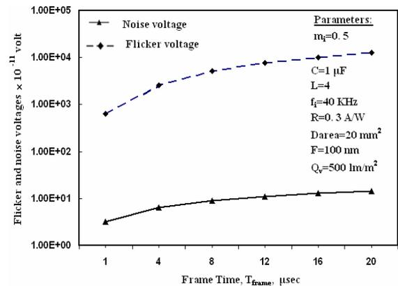
Fig.9 Effect of frame time for fluorescent lighting.
