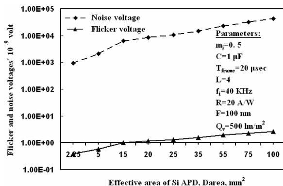
Fig.14 Effect of photodiode effective area for Si APDs for fluorescent lighting.
