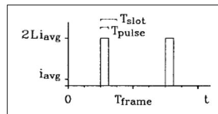
Fig.1. PPM modulation scheme [3].
