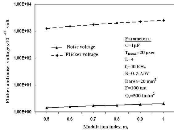
Fig.7 Effect of modulation index for fluorescent lighting.
