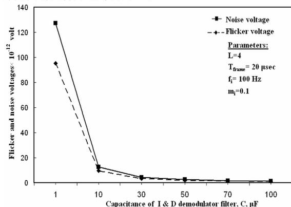
Fig.4 Effect of demodulator capacitance for incandescent lighting
