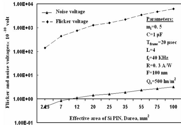
Fig.12 Effect of photodiode effective area for Si p-i-n photodiodes for fluorescent lighting.
