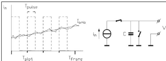
Fig.2 Signals at the receiver input and the schematic of the I&D demodulator filter [3].
