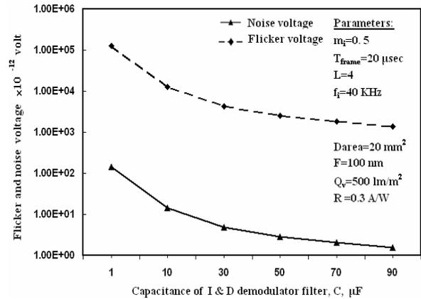
Fig.8 Effect of demodulator capacitance for fluorescent lighting
