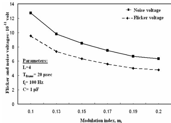
Fig.3 Effect of modulation index for incandescent lighting.
