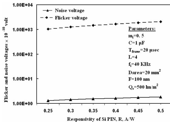
Fig.11 Effect of responsivity for Si p-i-n photodiodes for fluorescent lighting.
