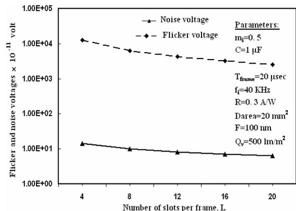
Fig.10 Effect of number of slots per frame for fluorescent lighting
