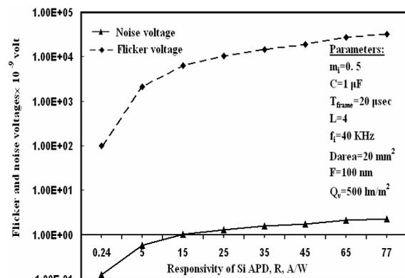
Fig. 13 Effect of responsivity for Si APDs for fluorescent lighting.
