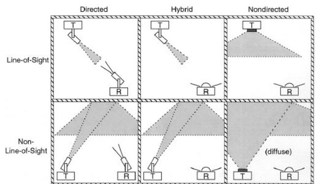
Fig. 1 Classification of simple infrared LOS and non-LOS links [2].
