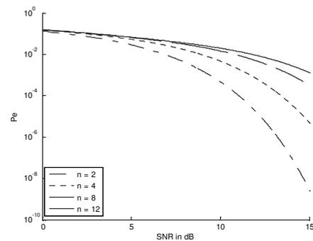
Fig. 5 Probability of error vs signal to noise ratio in diffused environment.
