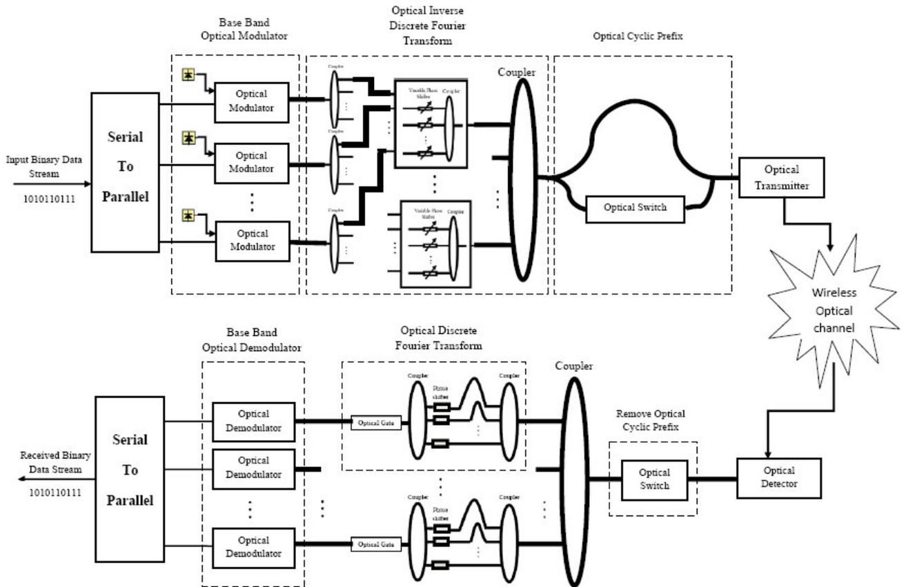
Fig. 2 Complete system architecture of all optical OFDM .
