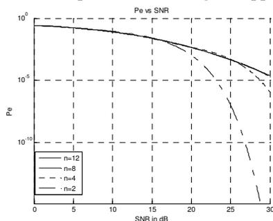
Fig. 6 Probability of error vs signal to noise ratio in LOS environment.
